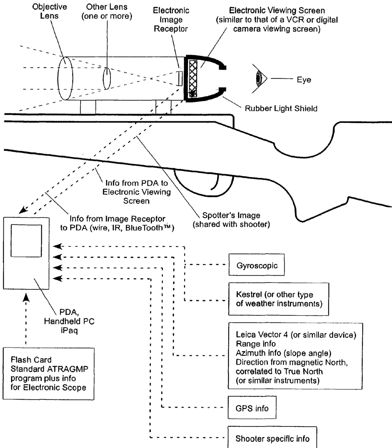
Electronic Target Acquisition Device
