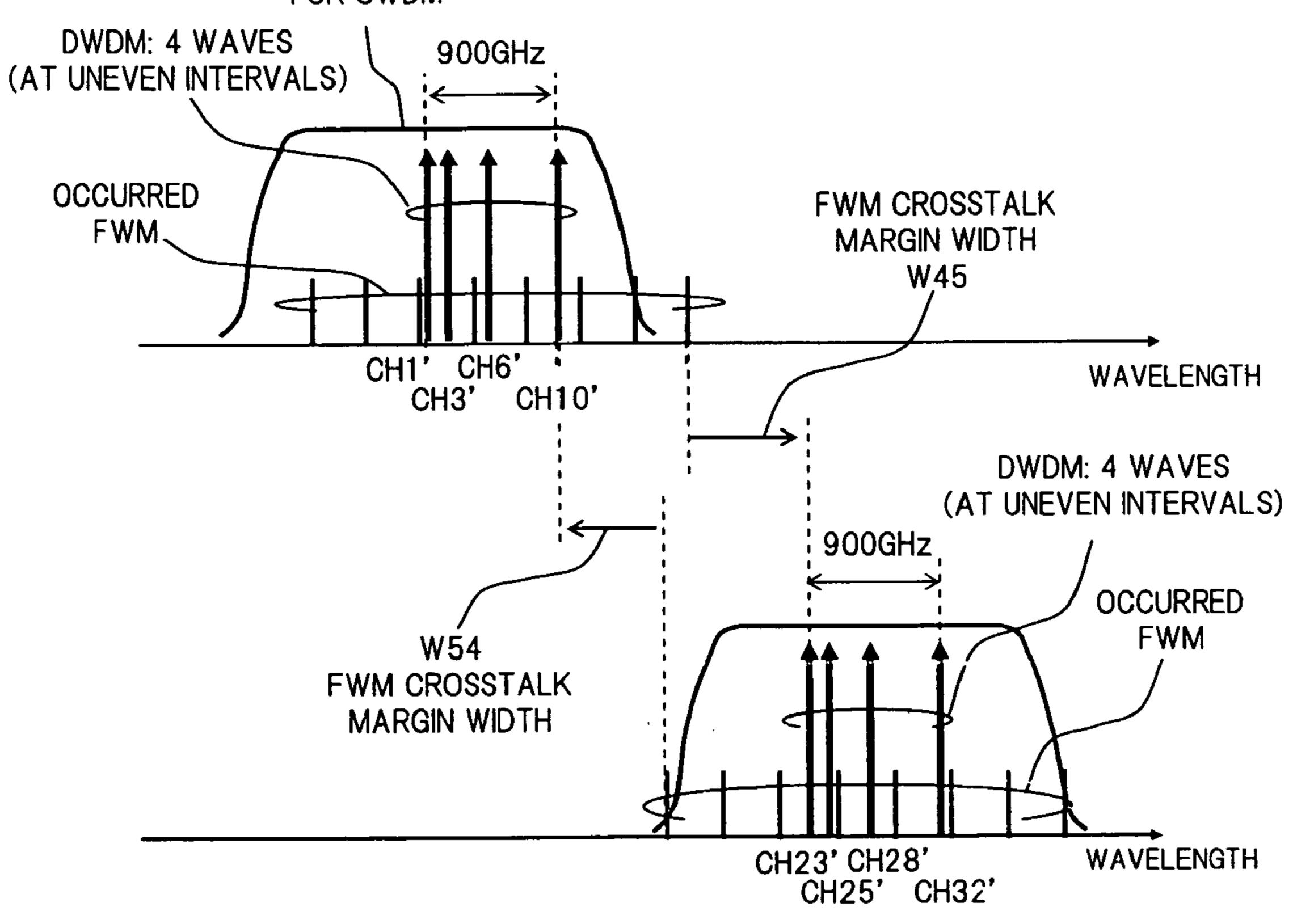
DWDM SIGNAL ARRANGEMENT IN 1550nm BAND
