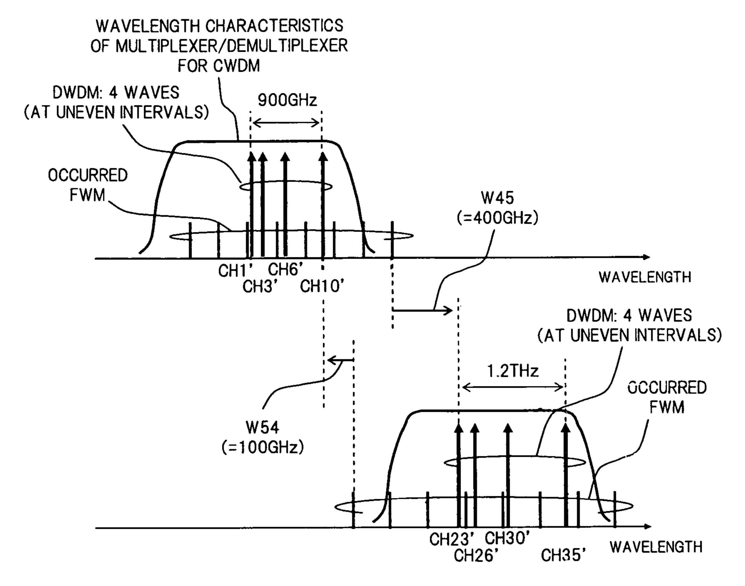
DWDM SIGNAL ARRANGEMENT IN 1550nm BAND
