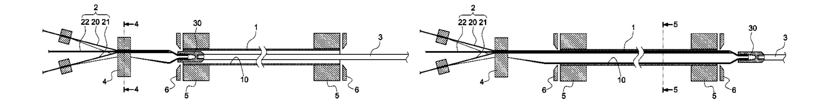
providing two elongated stripe-like continuous woven meshes, a plurality of fibers and a heat pipe body for accommodating the two woven meshes and the fibers;
