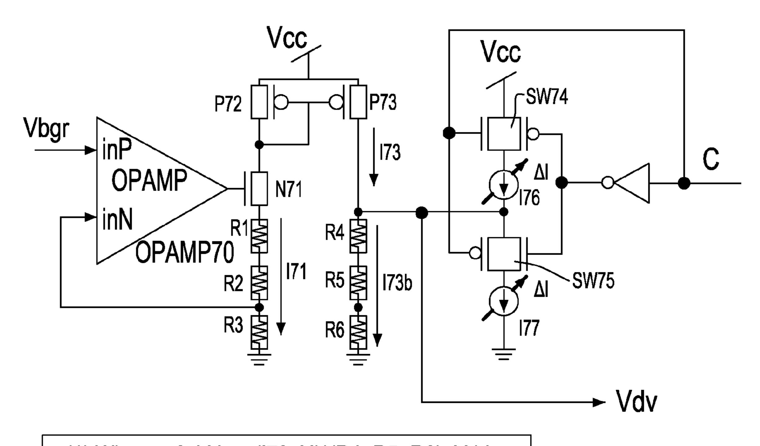
(1) When c=0,  $Vdv = (I73-\Delta I)*(R4+R5+R6)=Vdd$ (2) When c=1,  $Vdv = (I73+\Delta I)*(R4+R5+R6) = Vdd'$ Where, I71 = I73 = Vbgr/R3
