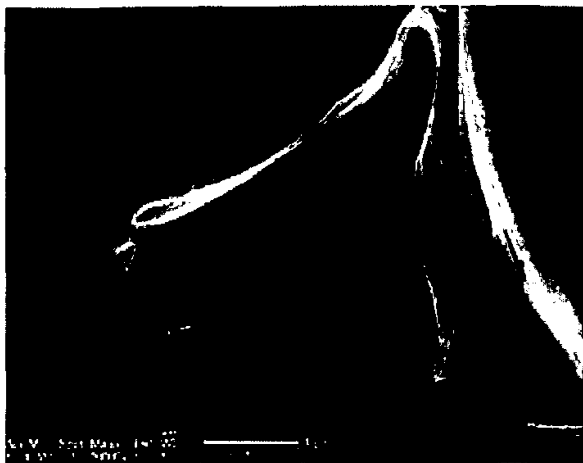
Fig. 13D: Sample: A9A-2: Fracture surface of pore wall
