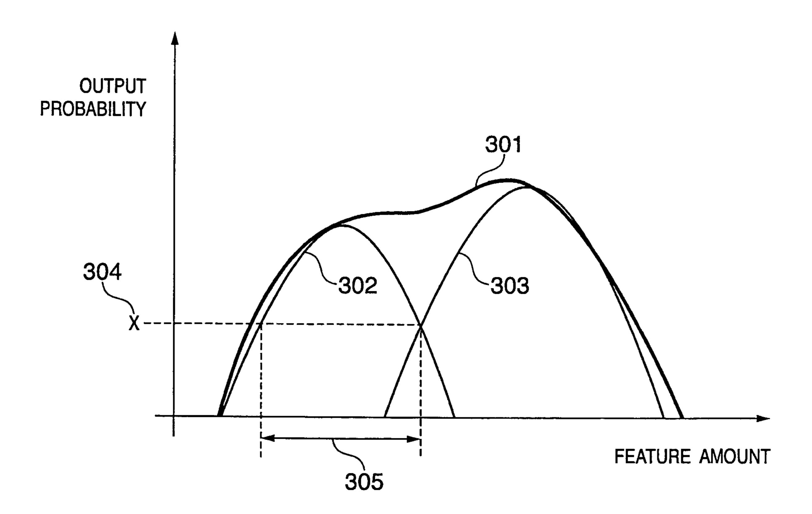
CALCULATING METHOD (3) FOR LOGARITHMIC OUTPUT PROBABILITY B OF STATE s FOR OBSERVATION SIGNAL O (1)
