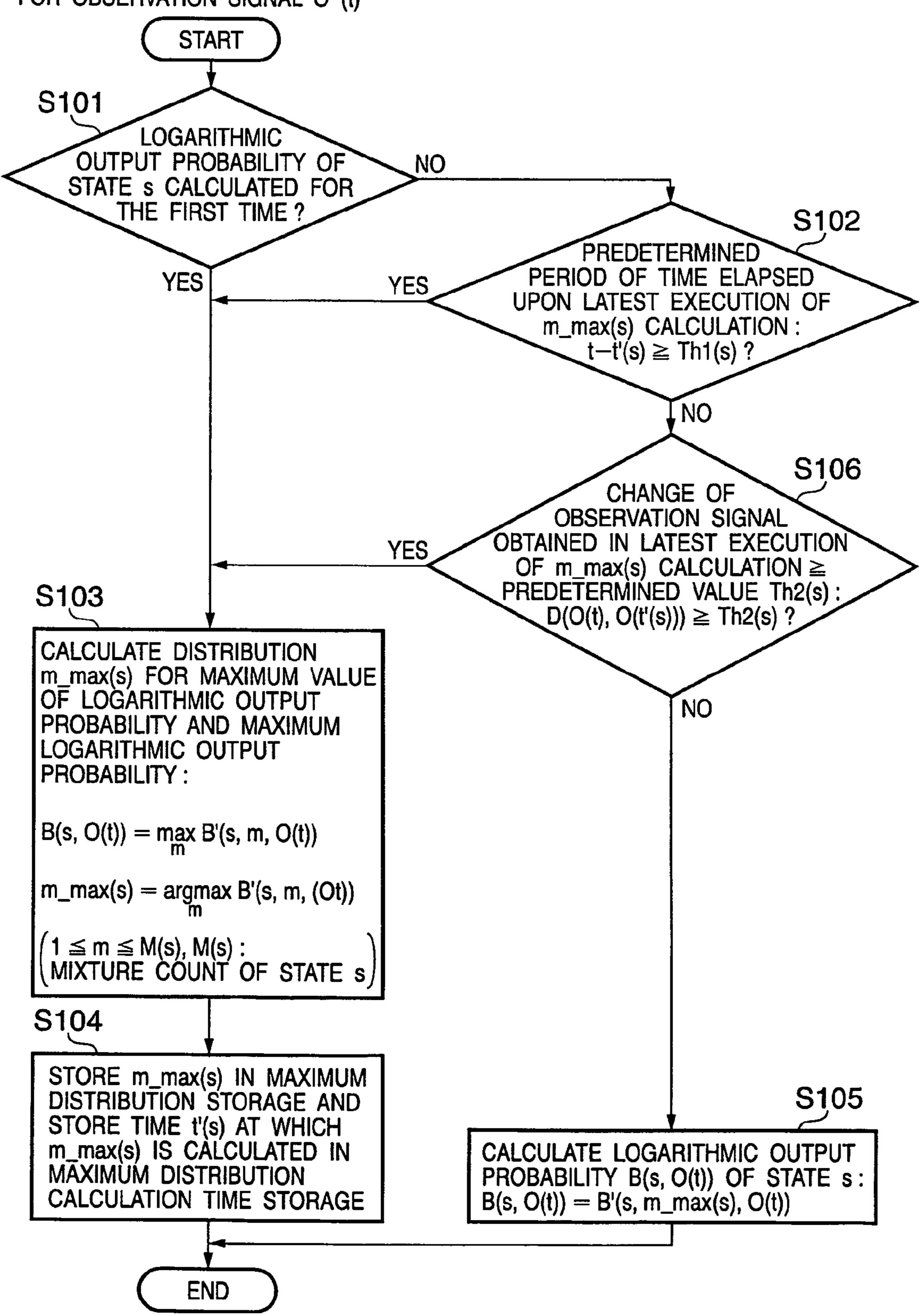
CALCULATING METHOD (5) FOR LOGARITHMIC OUTPUT PROBABILITY B OF STATE S FOR OBSERVATION SIGNAL O (t)
