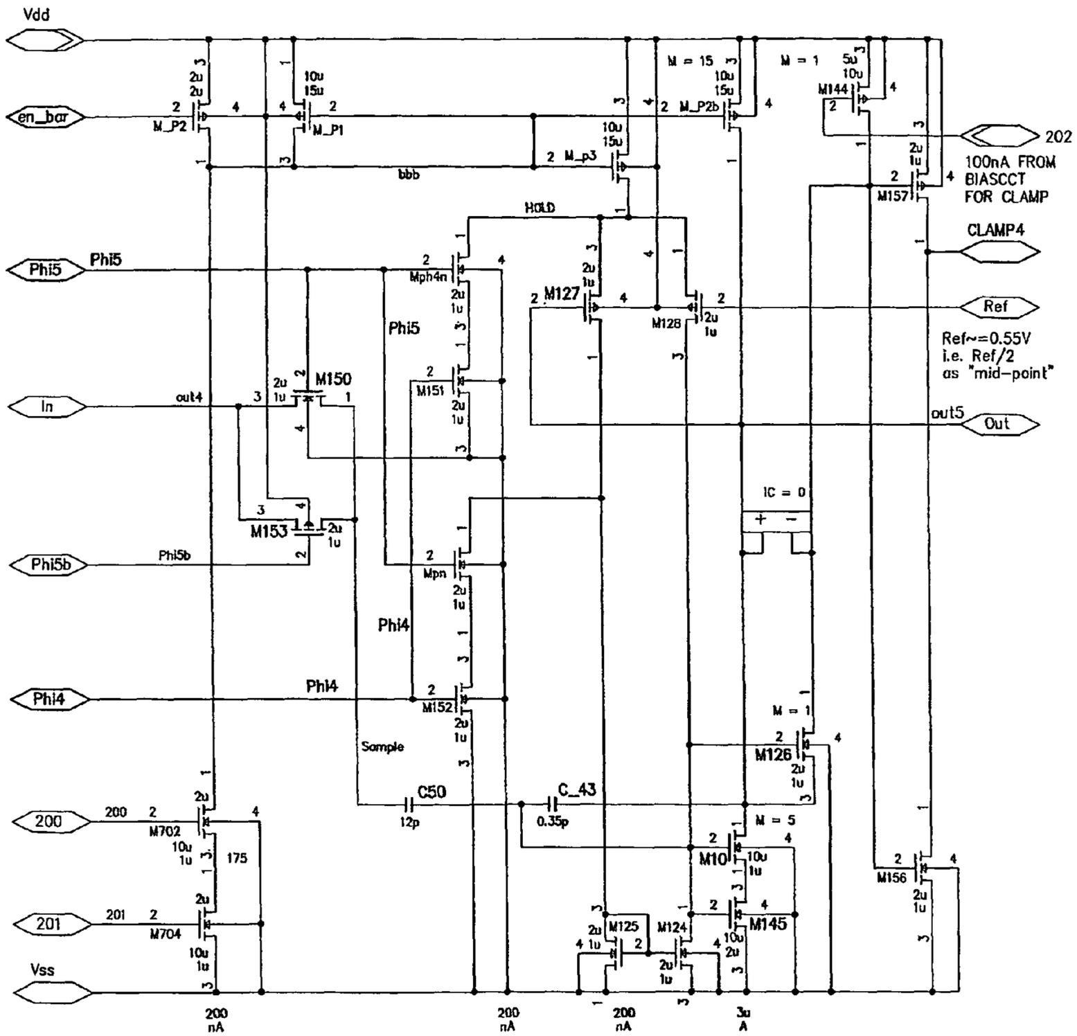
Note: For 1st & 2nd Stage, all cap are drawn on top of Vdd-connected N-well
