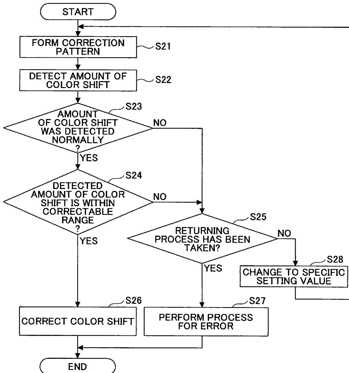
**COLOR SHIFT CORRECTING APPARATUS
