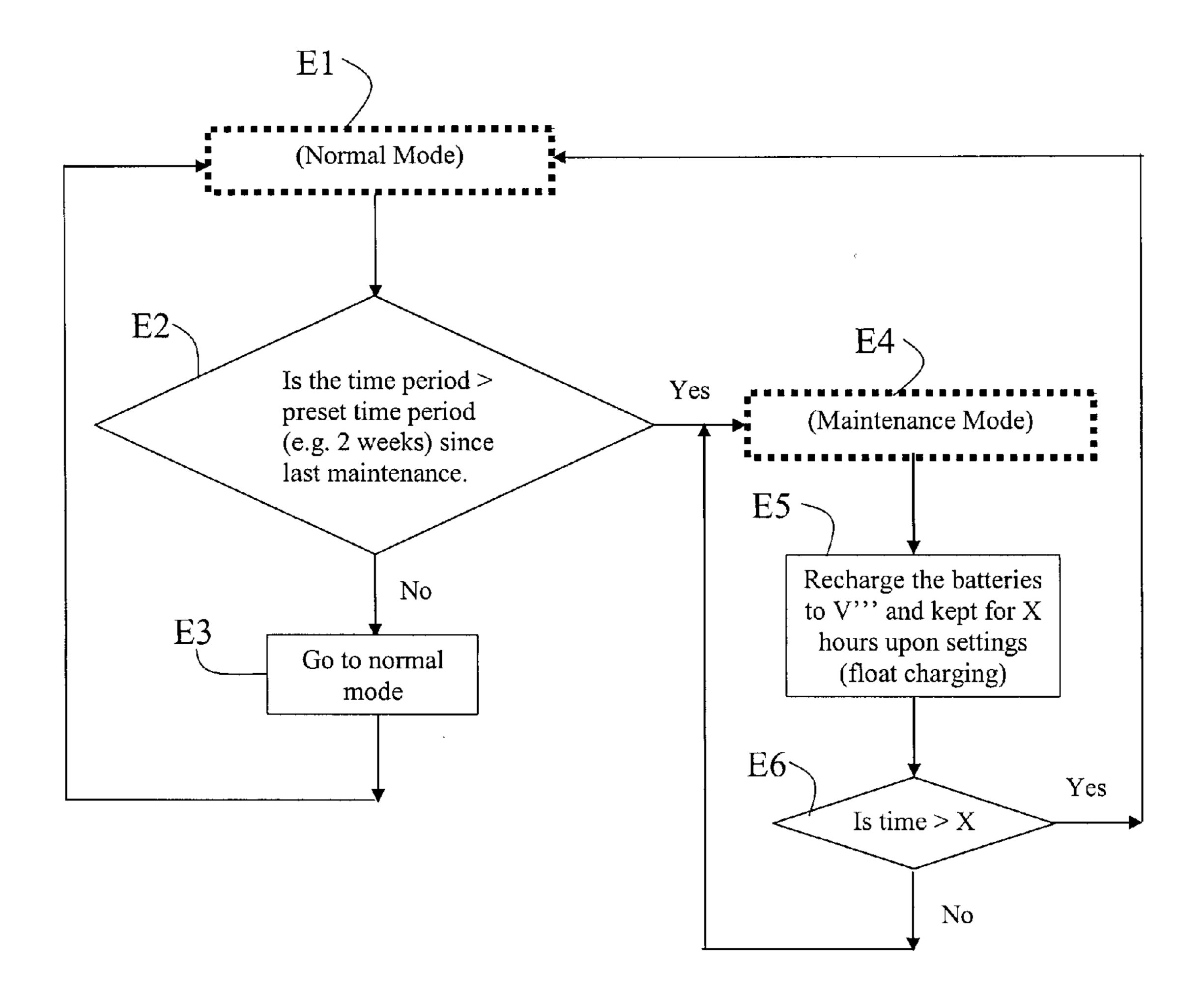
V = V oltage detected from battery module. V''' = O ne preset voltage value designated for float charging.
