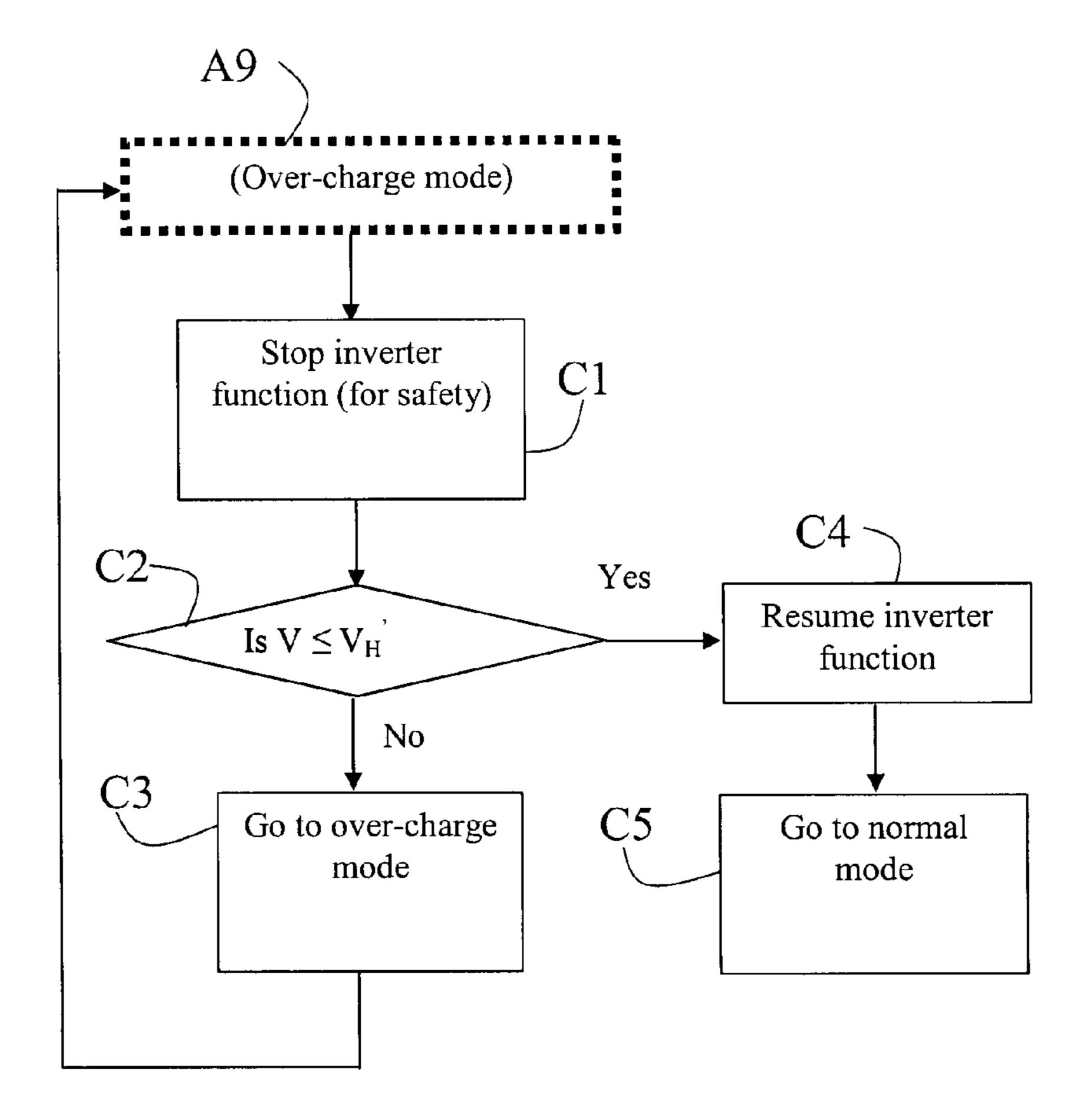
V = Voltage detected from battery module.  $V_{H} = One preset high voltage value that terminates the over-charge mode.$
