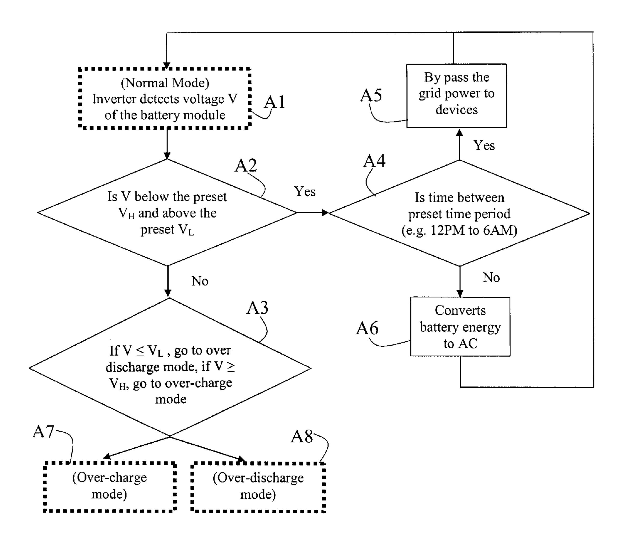
V = Voltage detected from battery module.
