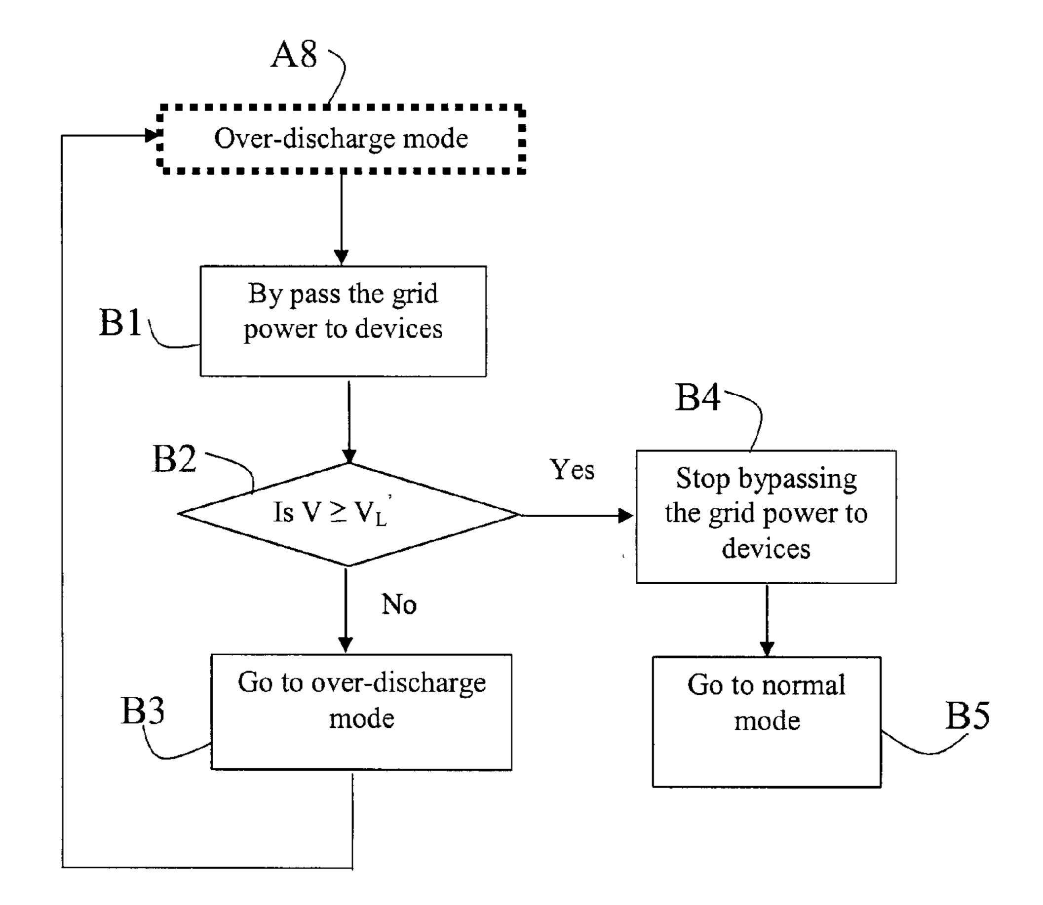
√ = Voltage detected from battery module.
