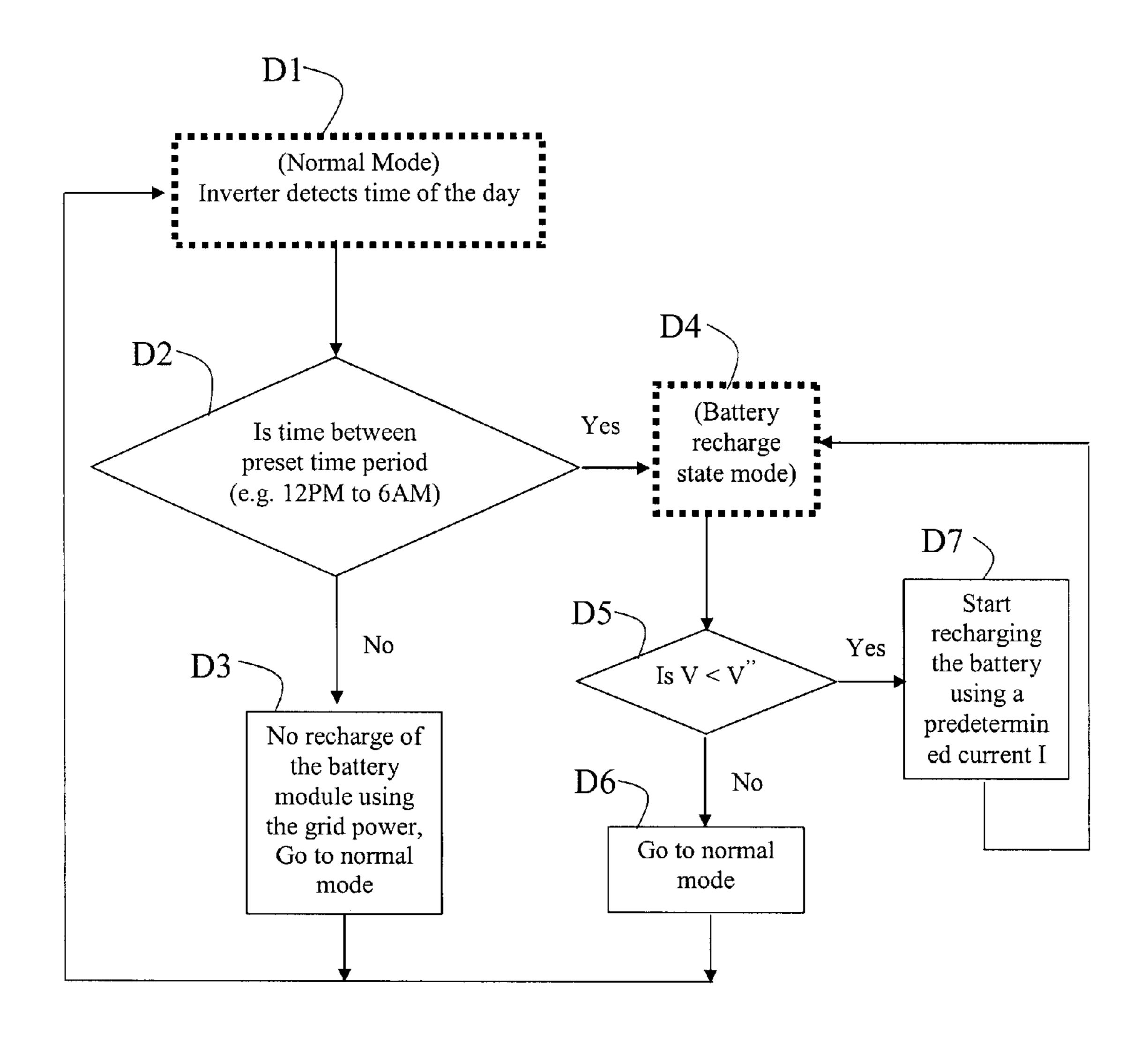
V = Voltage detected from battery module. V" = One preset voltage value that determines how much capacity to be recharged. This voltage is designed according to the season change.
