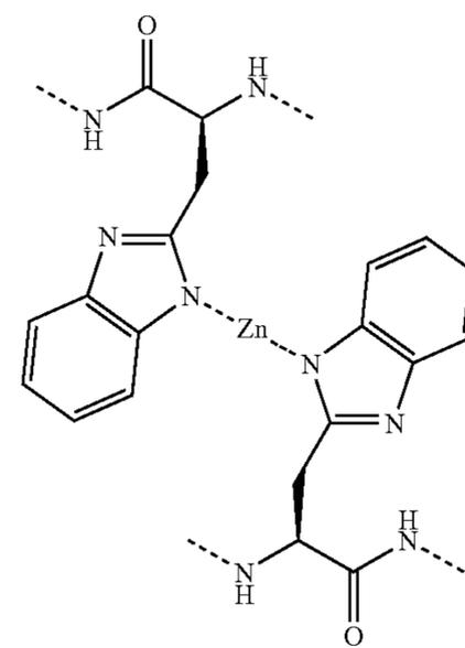
Scheme 3 above illustrates the reaction of an aqueous zinc (II) ion (e.g. from zinc chloride or zinc acetate) with two equivalents of an appropriate imidazole (e.g. benzimidazole) to form a zinc-benzimidazole complex.
