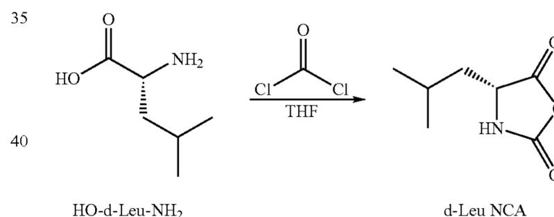
Synthesis of d-Leu NCA—d-Leu NCA was synthesized as described in Example 1 from HO-d-Leu-NH<sub>2</sub> (20.0 g, 152.5 mmol) and 99.3 mL (198.3 mmol) of phosgene (20% in toluene). 13.8 g (58% yield) of NCA was isolated as a white, crystalline solid. <sup>1</sup>H NMR (d<sub>6</sub>-DMSO) δ 9.13 (1H), 4.44 (1H), 1.74 (1H), 1.55 (2H), 0.90 (6H) ppm.
