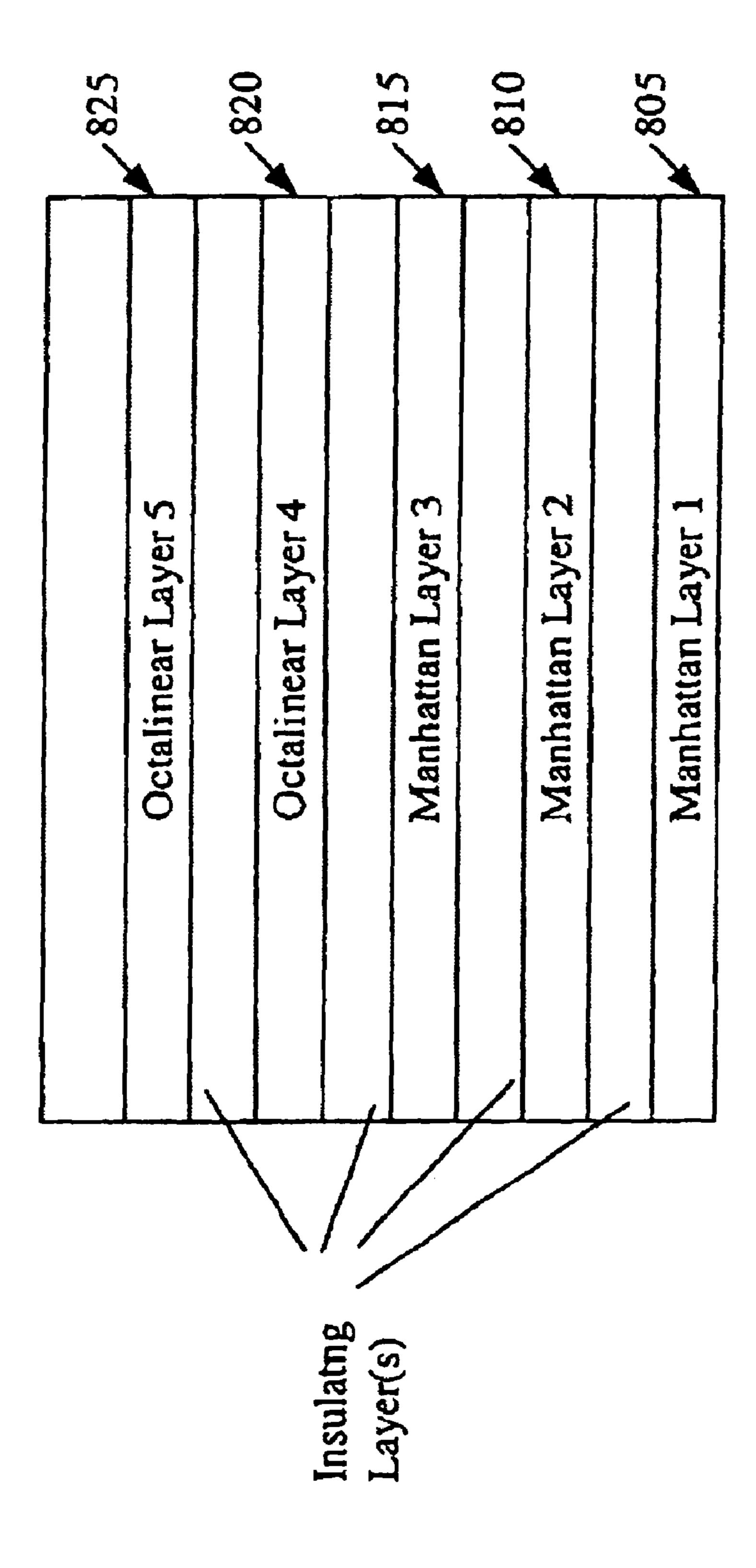
Fig. 2 - Layers with Different Routing Directions
