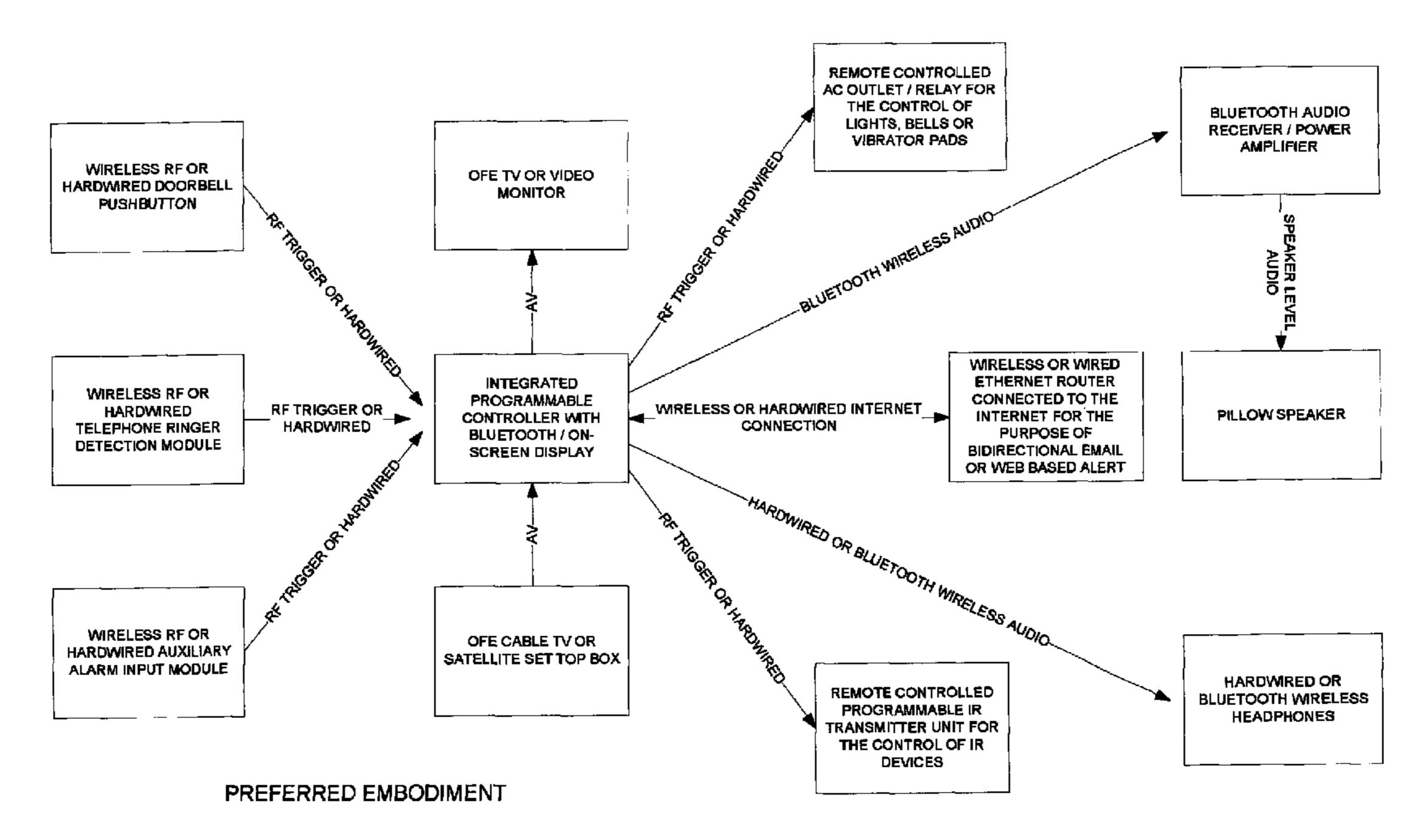
An Integrated Programmable Controller with Bluetooth audio / on-screen video display capability that accepts both hardwired and wireless RF triggers that result in interrupts of audio and video signals then displaying the cause of the interrupt in on-screen video and amplified audio at a remote location for the primary purpose of assisting a hearing or visually impaired individual or just someone who wants to view television without disturbing anyone around them.
