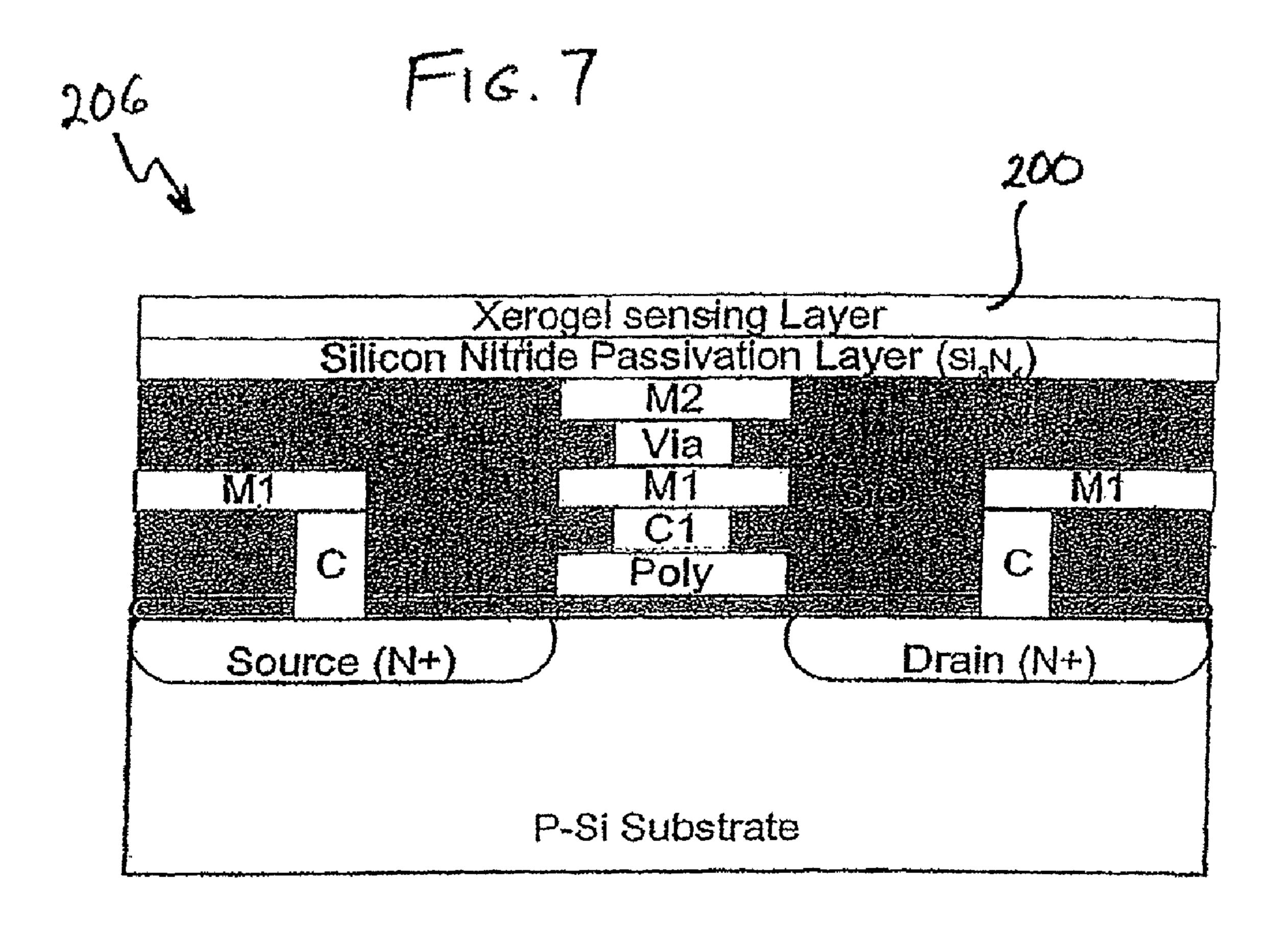
C: Active contact, CI: Poly contact, MI: metal I layer, M2: metal 2 layer, Via: Metal I to Metal 2 connection
