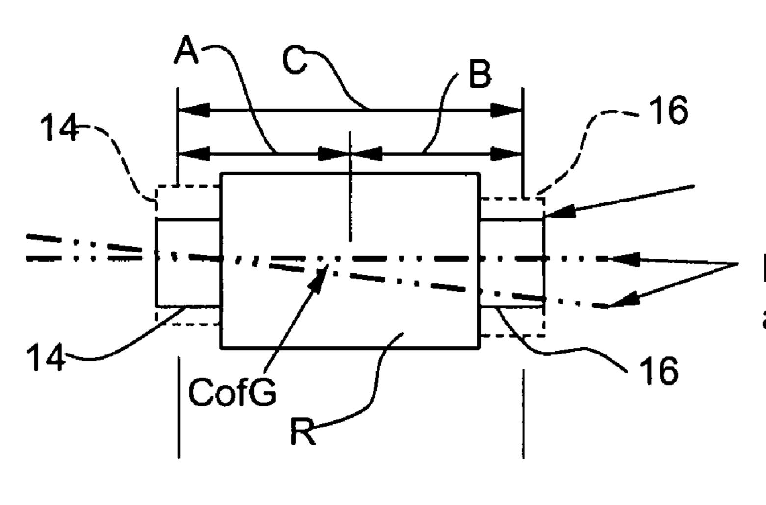
Rotational axes before and after correction
