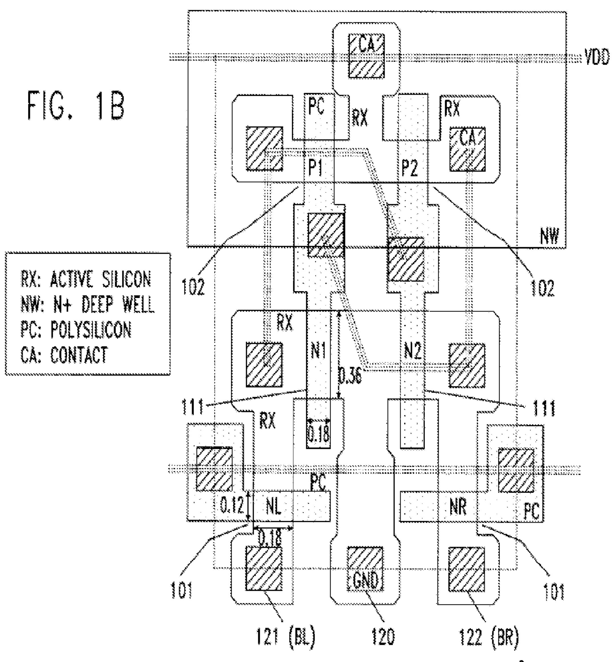
CONVENTIONAL 6-T SRAM CELL 1.35 X 1.96 = 2.65  $\mu$ m<sup>2</sup> 0.13 $\mu$ m CMOS, beto = 2
