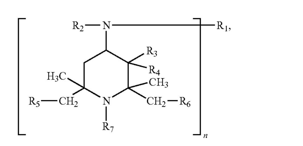
wherein the general symbols are as defined in claim 1, as stabilizers for protecting organic materials, in particular synthetic polymers, against oxidative, thermal, dynamic, light-induced and/or ozone-induced degradation.
