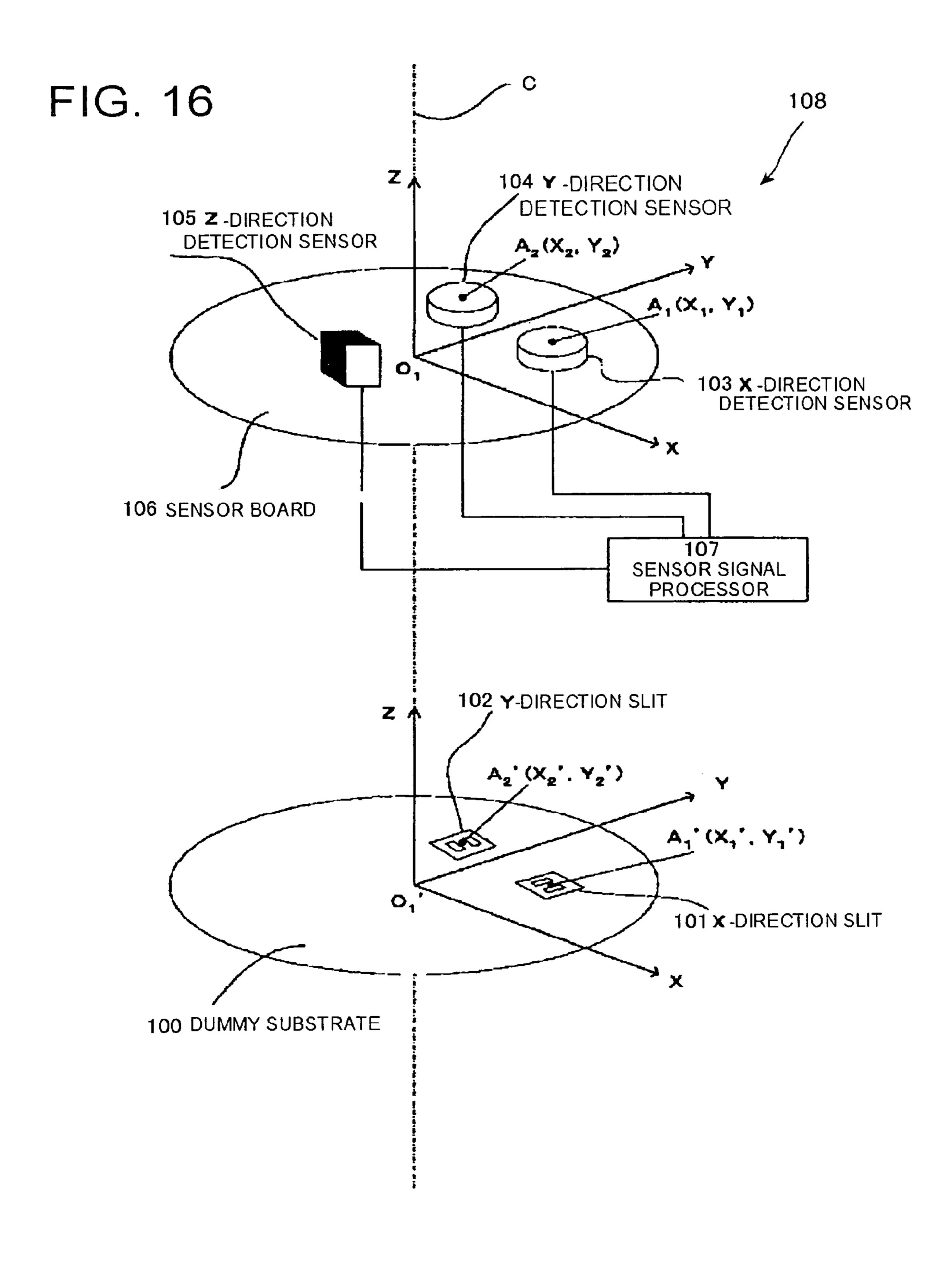
TEACHING APPARATUS AND METHOD OF TEACHING A WAFER CARRYING APPARATUS A TARGET POSITION FOR PLACING AND REMOVING SEMICONDUCTOR WAFERS ON AND OFF A WAFER BOAT USING AN IMAGING DEVICE AND DISTANCE SENSOR
