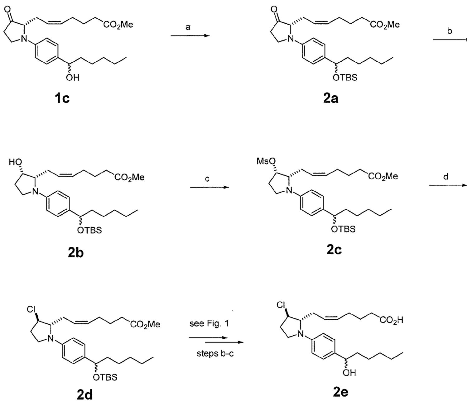
(a) TBSOTf, Et<sub>3</sub>N, CH<sub>2</sub>Cl<sub>2</sub>; (b) L-Selectride, THF; (c) MsCl, Et<sub>3</sub>N, CH<sub>2</sub>Cl<sub>2</sub>; (d) TBAC, toluene.
