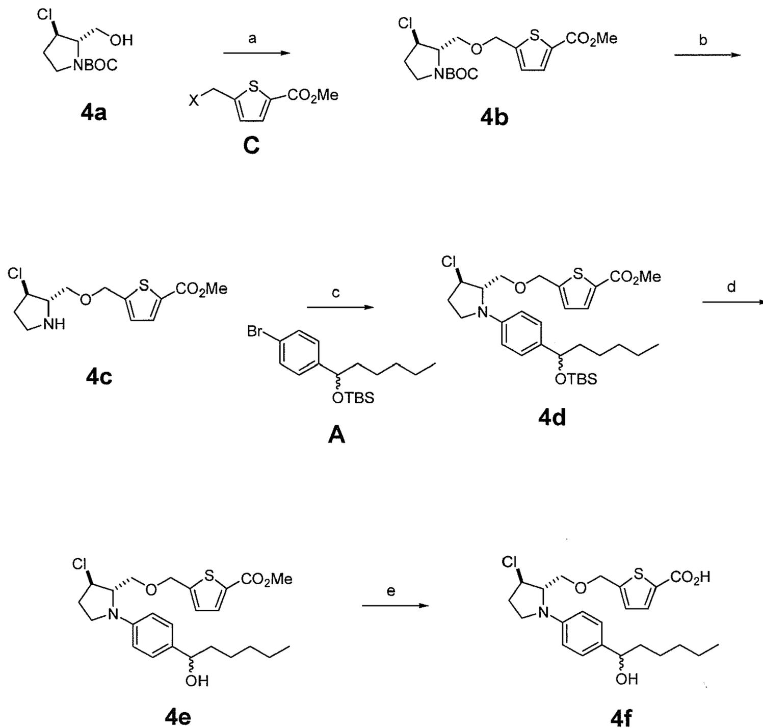
(a) NaH, A, DMF; (b) 3M HCl in dioxane; (c) B, Pd(0), ligand, base, solvent; (d) HF-pyridine, MeCN; (e) LiOH, H<sub>2</sub>O, THF.
