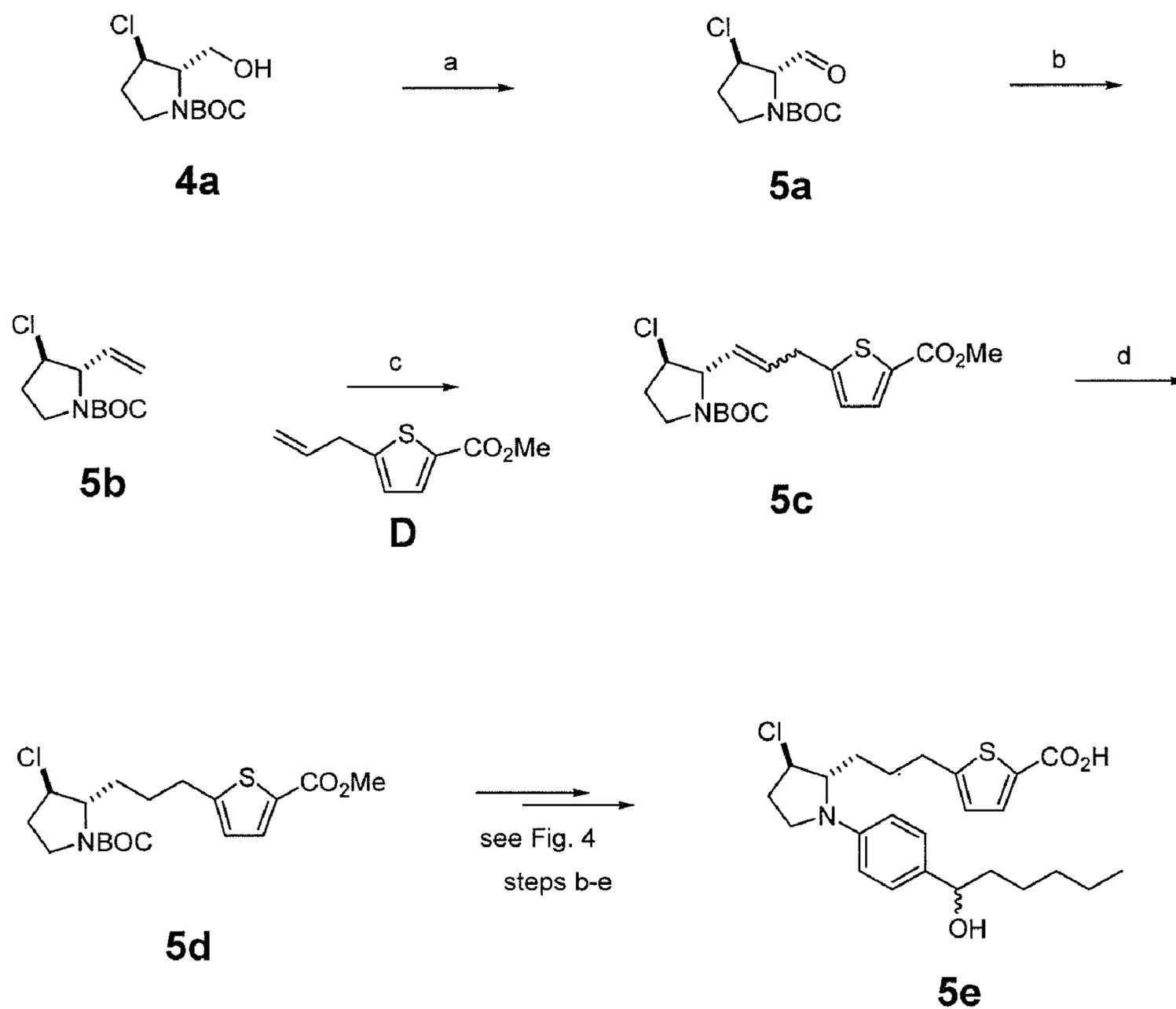
(a) Swern oxidation; (b) Tebbe methylenation; (c) **C**, Grubbs' 2nd generation catalyst,  $\text{CH}_2\text{Cl}_2$ ; (d)  $\text{H}_2$ , Pd/C, EtOAc.
