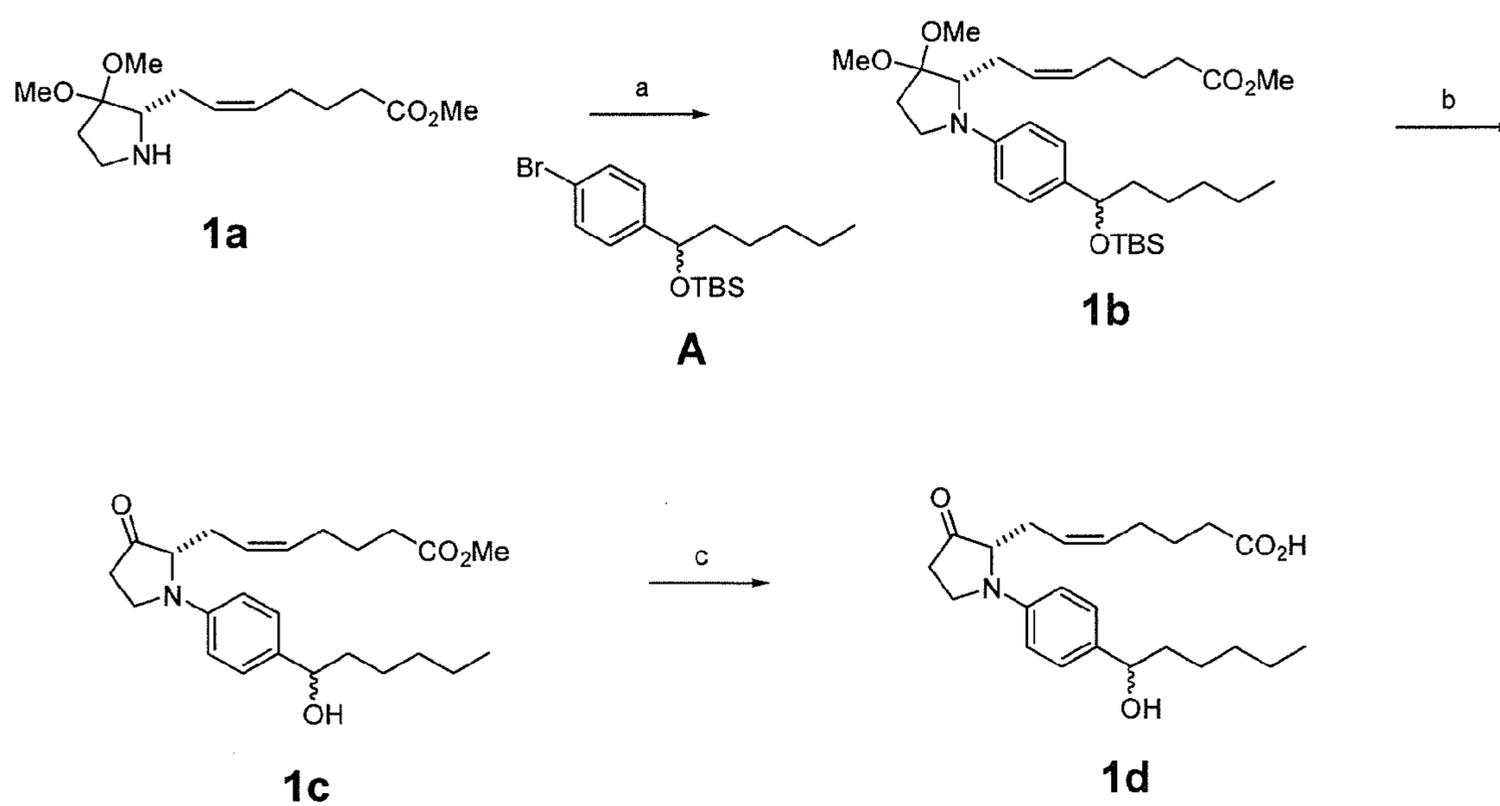
(a) B, Pd(0), ligand, base, solvent; (b) 6M HCl in dioxane; (c) LiOH, H<sub>2</sub>O, THF.
