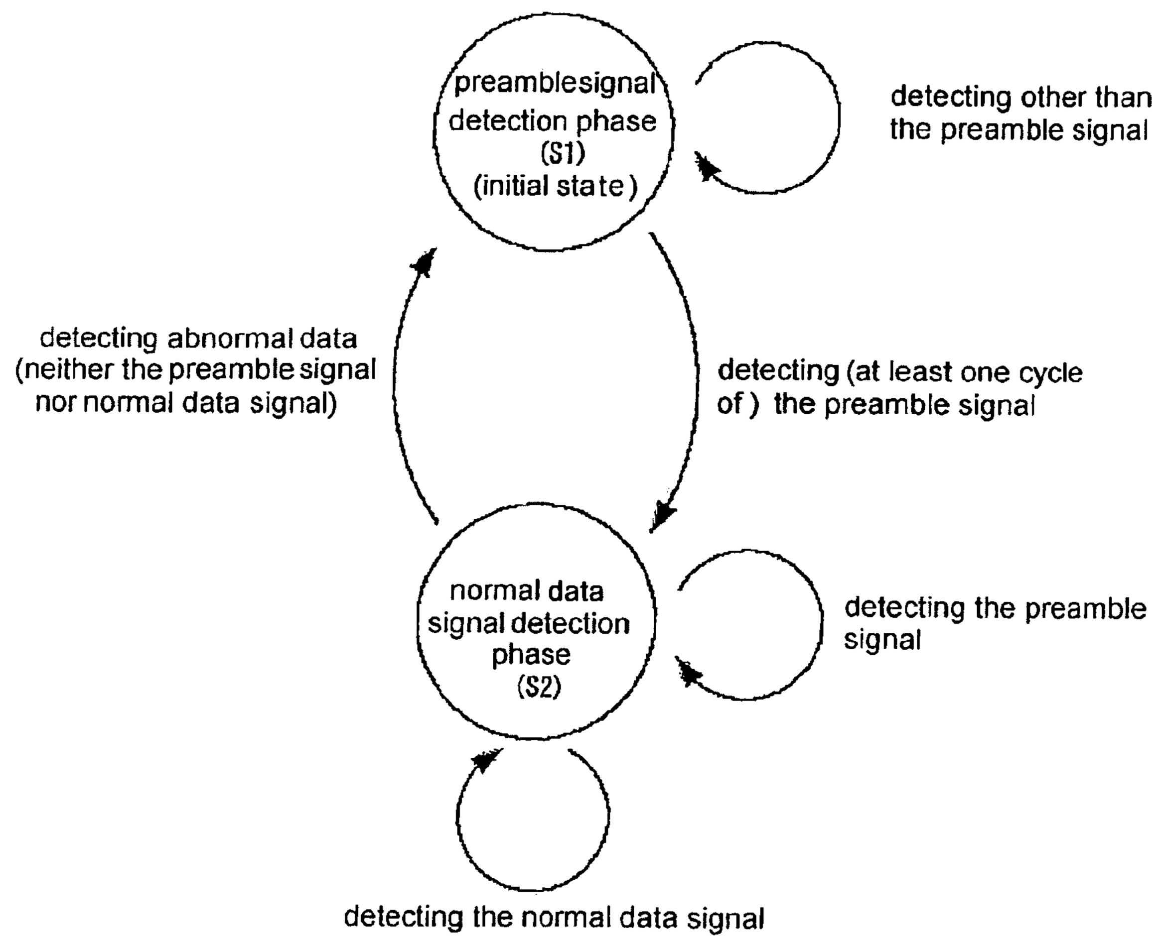
detecting the normal data signal →outputting the data to the buffer circuit
