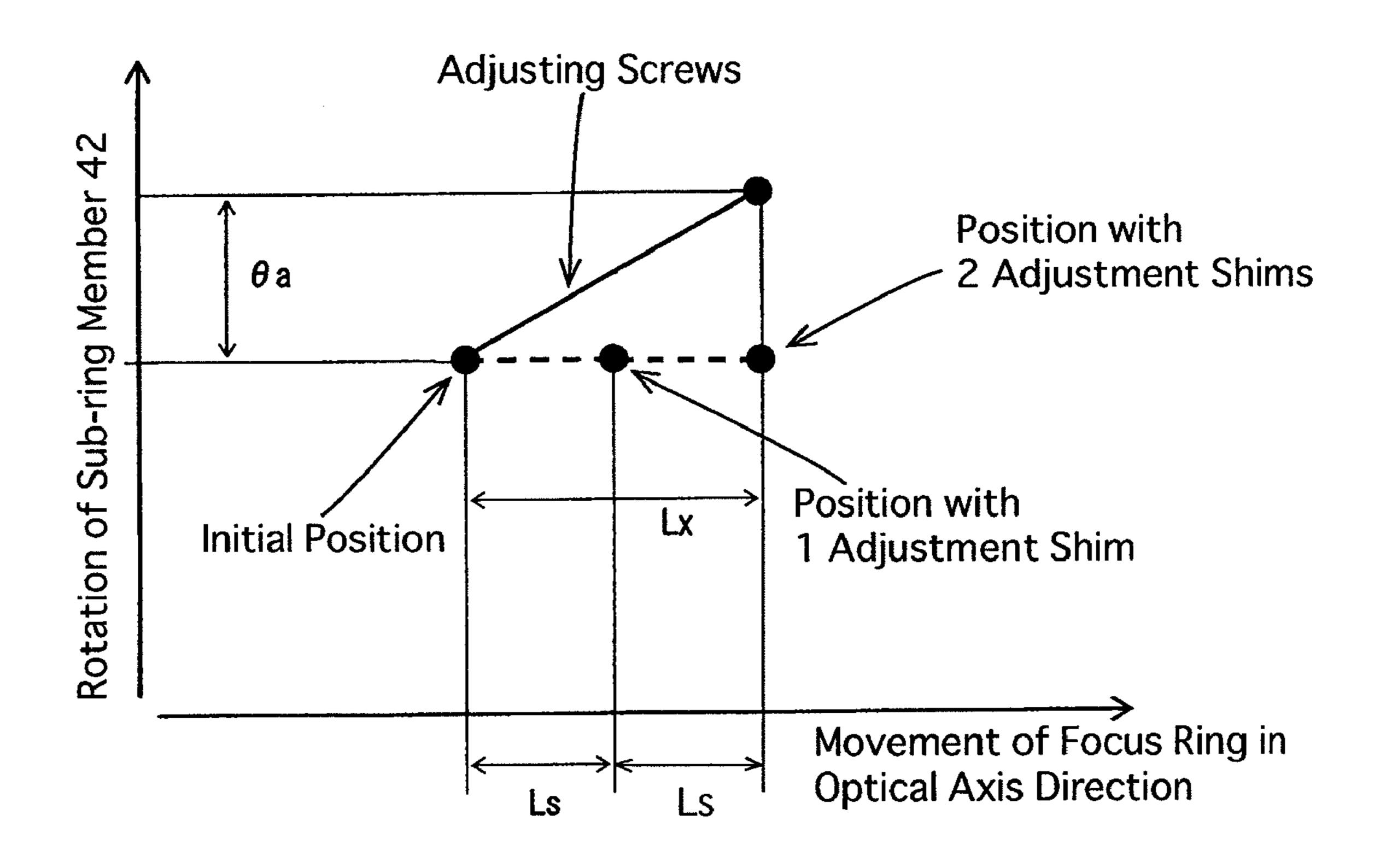
Ls: Movement Amount via 1 Adjustment Shim Lx: Movement Amount via Adjusting Screws
