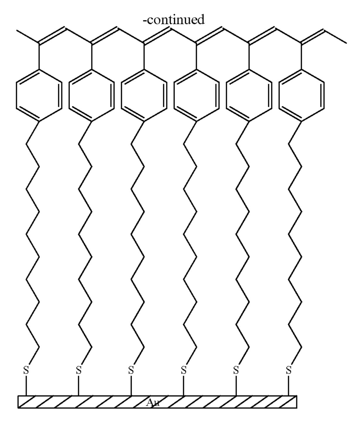
Example 3, above, illustrates a SAM of alkylphenylacetylene on an oxide insulating layer that has been polymerized by dipping in a solution of a catalyst, for example, a Ziegler catalyst, to form polyphenylacetylene at the surface of a polymerized SAM, which may form an intramolecular charge transport pathway between source and drain electrodes of a field-effect transistor.
