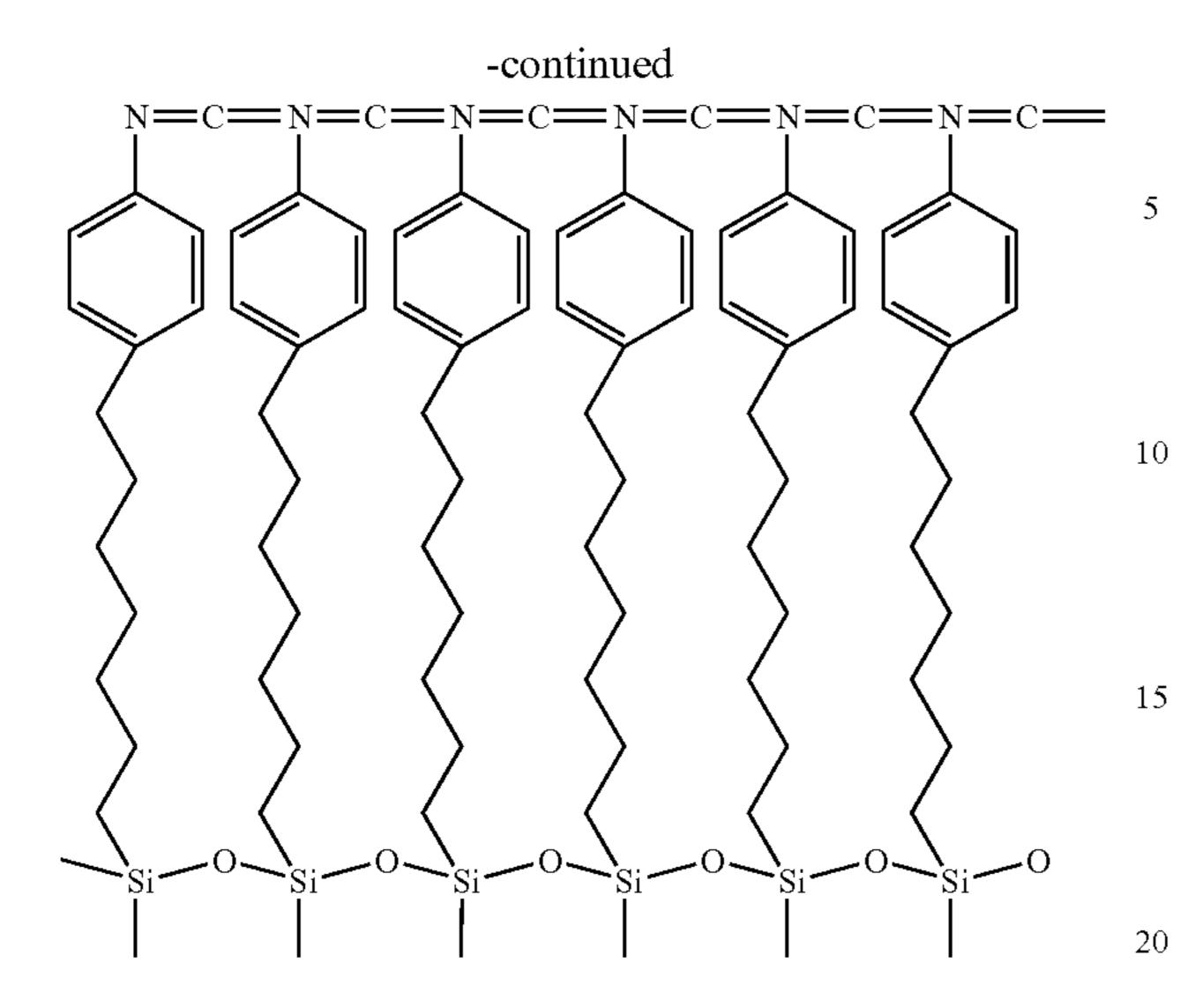
Example 2, above, illustrates a thermally induced polymerization of an end-cap functionality of isonitrile in a bifunctional molecule to form a polymerized SAM, which may be disposed on a substrate surface located between the source and drain electrodes of a field-effect transistor. This polymerized SAM includes an intramolecular charge transport pathway through the conjugated bonds, which forms a highly conductive pathway from one end to the other end of the polymerized SAM.
