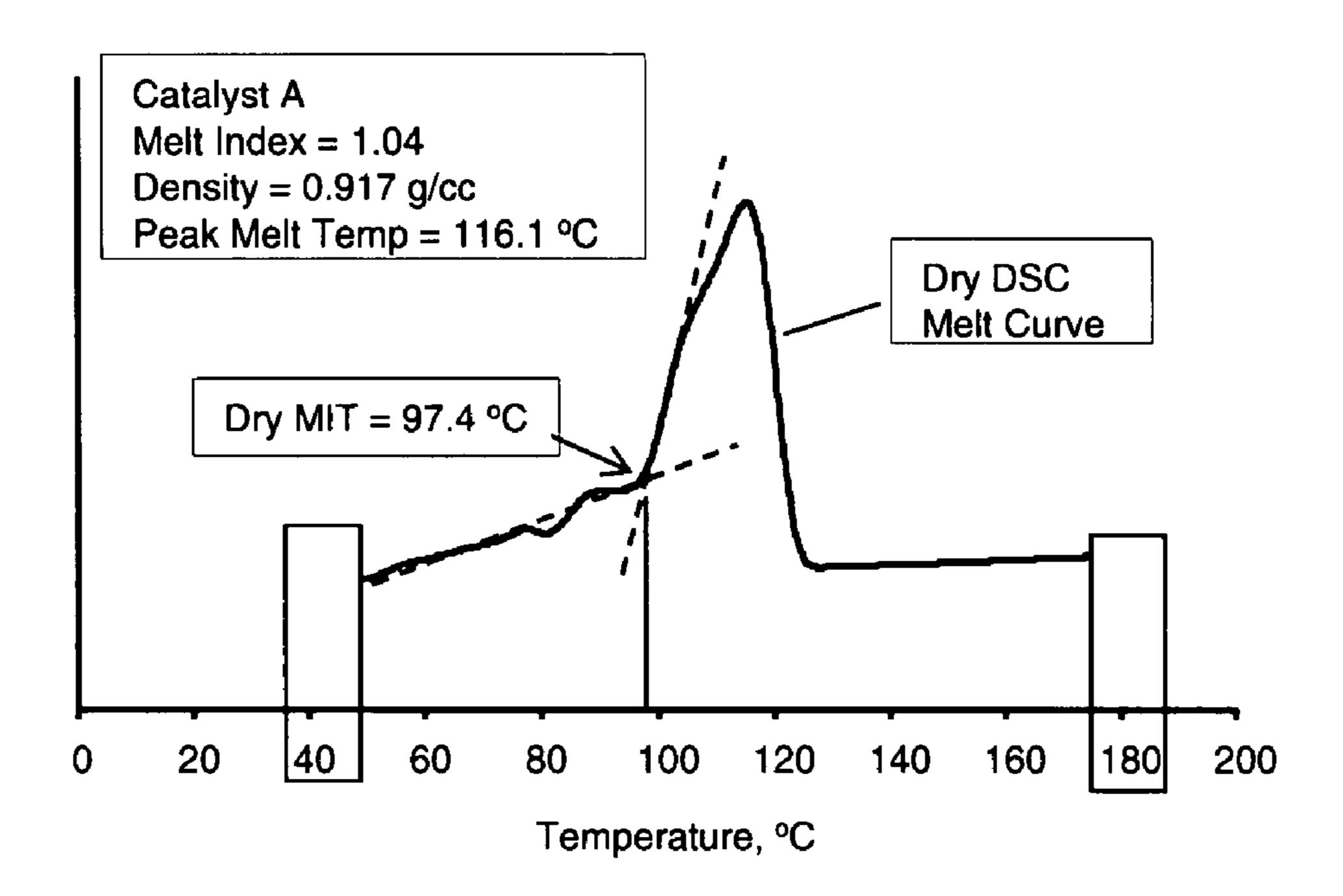
Figure 4 – Displaced MIT (MIT<sub>R</sub>)
