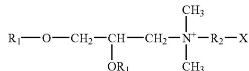
in which R<sub>1</sub> is a saturated or unsaturated straight-chain aliphatic radical having 12 to 18 carbon atoms, R<sub>2</sub> is another aliphatic radical containing 2 or 3 carbon atoms and X is an amine or hydroxyl group, e.g. the DMRIE. In another embodiment the cationic lipid can be associated with a neutral lipid, e.g. the DOPE.
