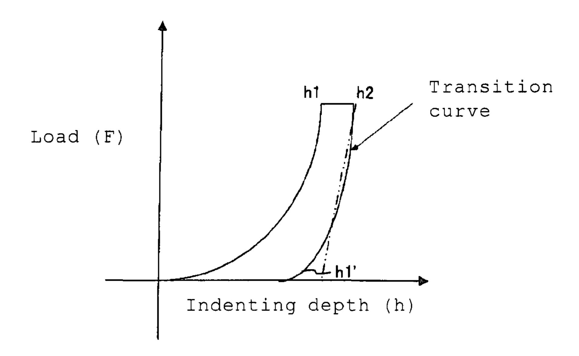
h1: depth when desired load is applied h2: state that h1 load is maintained h1': state that load is removed from
