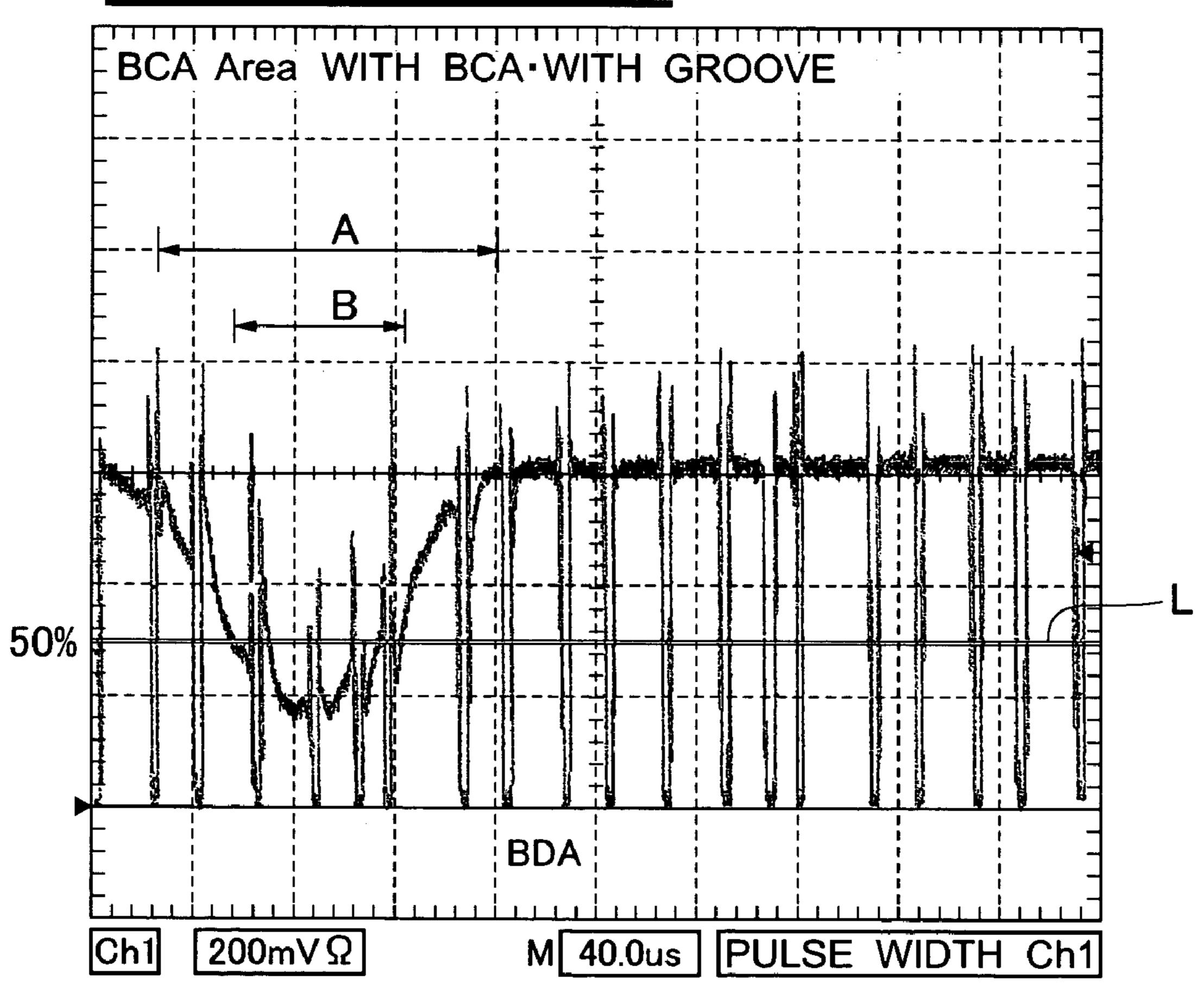
A:PORTION WHERE INTERFERENCE IS CAUSED BY GROOVES
