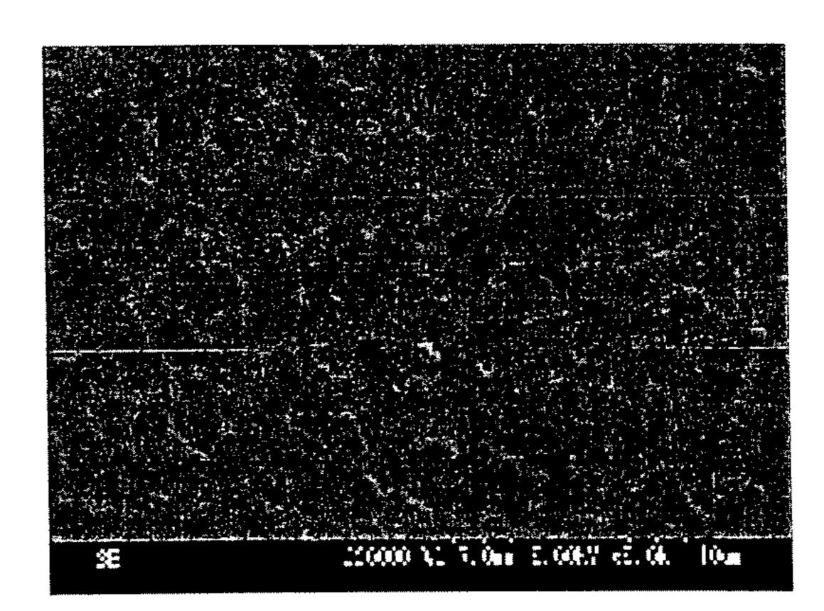
AMORPHOUS STRUCTURE (PEAK DIFFRACTION HALF WIDTH: GREATER THAN 1. 5°)
