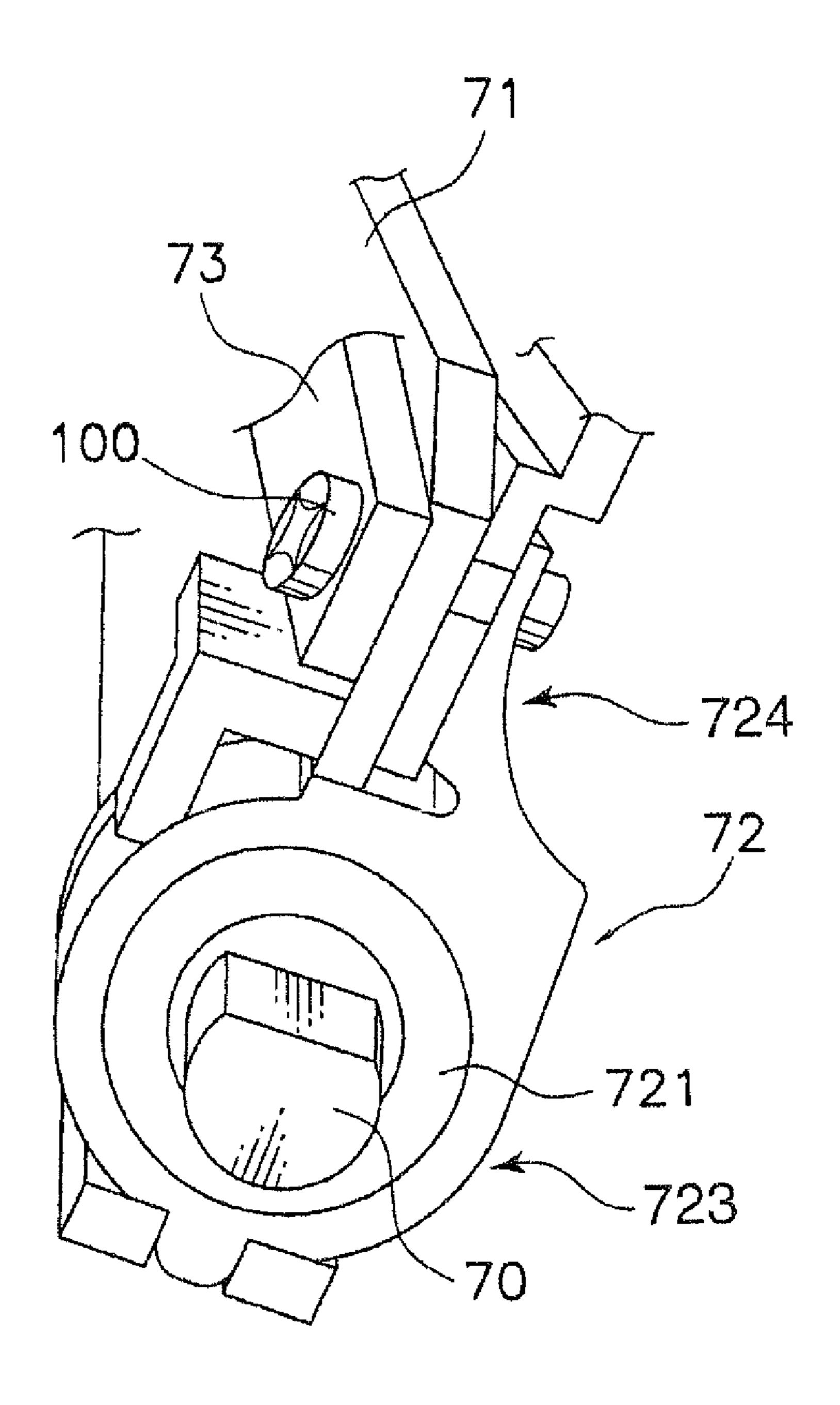
DEVELOPING DEVICE WITH STRUCTURE CONFIGURED TO REGULATE DISTANCE BETWEEN DEVELOPING ROLLER AND REGULATING MEMBER FOR DEVELOPER LAYER AND IMAGE FORMING APPARATUS WITH THE DEVELOPING DEVICE
