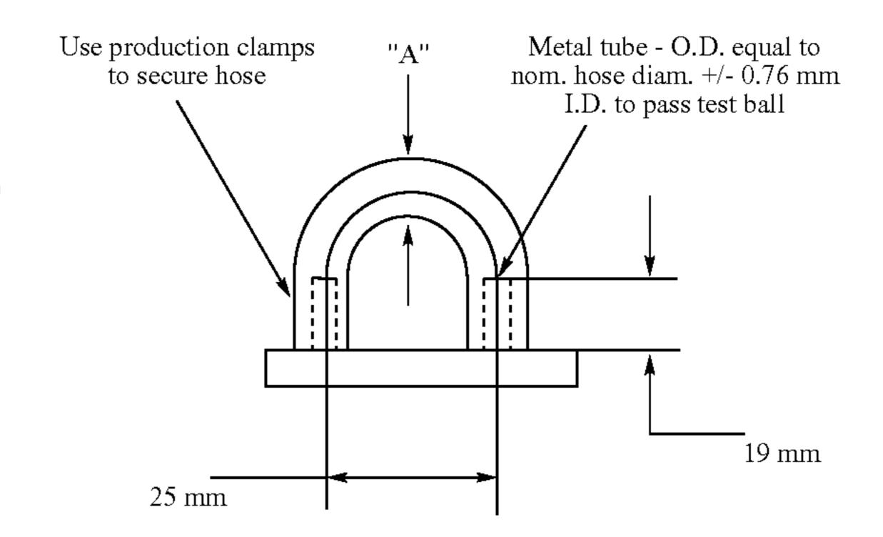
Sample Selection: Production hose selected for the kink test should represent, as nearly as possible, minimum wall thickness. When recording results include wall thickness, ovality, and dimension "A" (see above). This dimension is measured while sample is on the test fixture.
