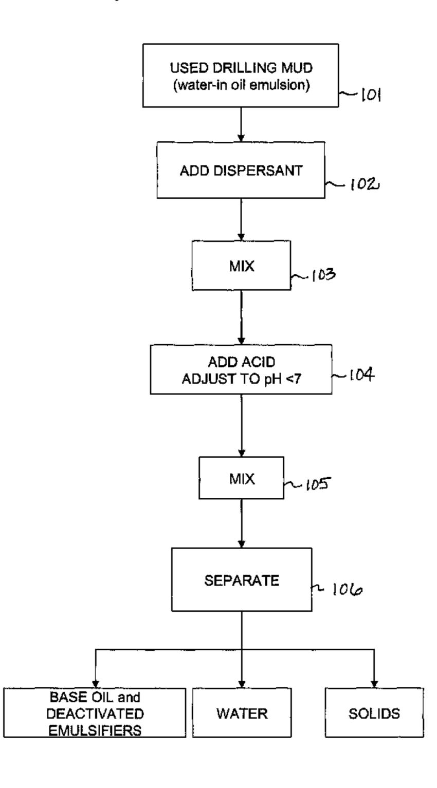
Fig. 1 USED DRILLING MUD (water-in oil emulsion) ~ 102 MIX ADD ACID -104 ADJUST TO pH <7 MIX SEPARATE 106 BASE OIL and DEACTIVATED WATER SOLIDS EMULSIFIERS
