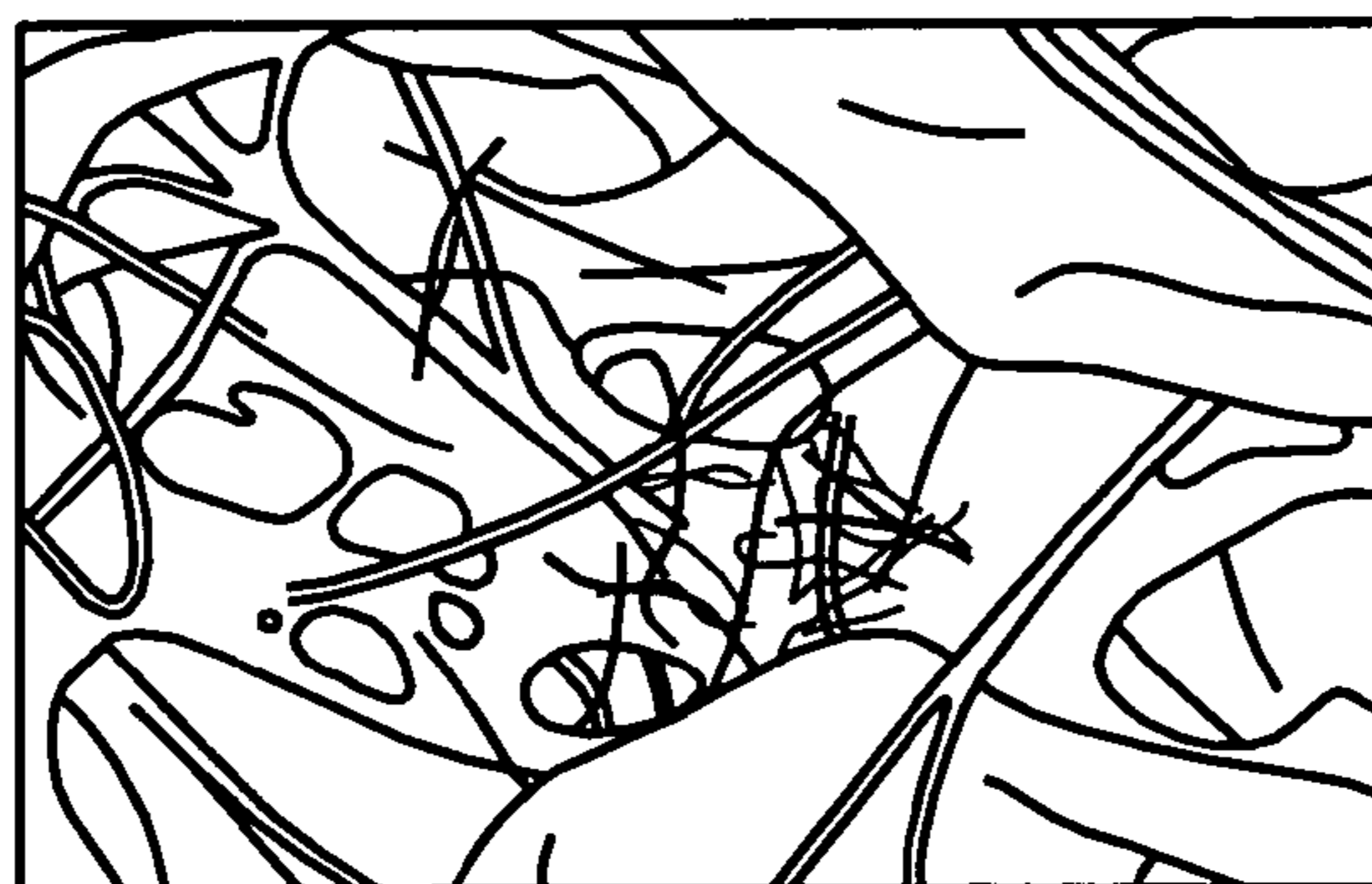
FIG. 20 COMMERCIAL FUEL GRADE CELLULOSE MEDIA CF PRIOR ART
