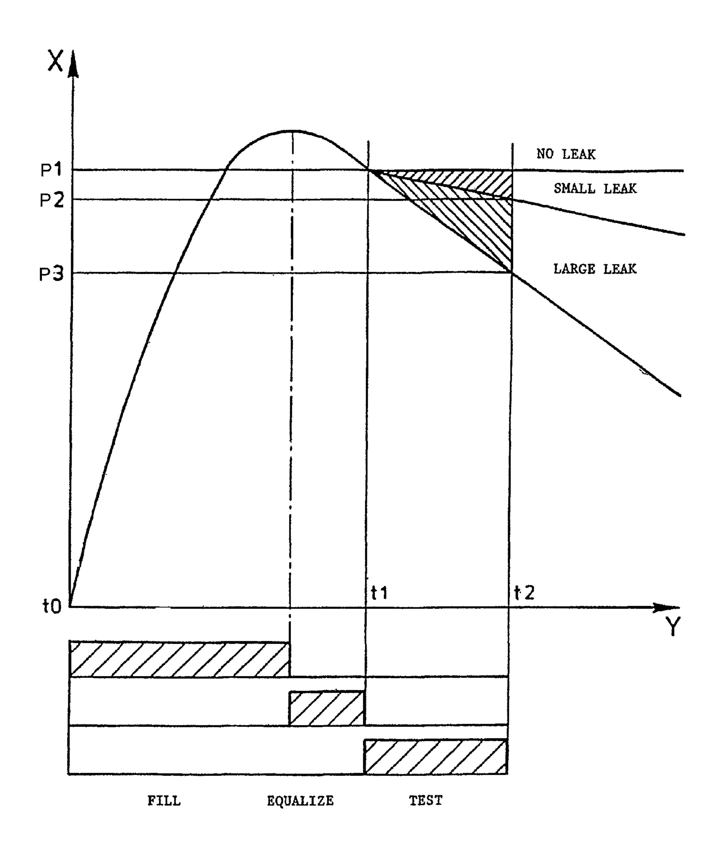
P1 CONVERTER VALUE AT MEASUREMENT POINT t1 FOR REFERENCE FORMATION CONVERTER VALUE AT MEASUREMENT POINT t2 FOR LEAK EVALUATION WITH CONTAINER HAVING NO LEAK (P1)/SMALL LEAK (P2)/LARGE LEAK (P3)
