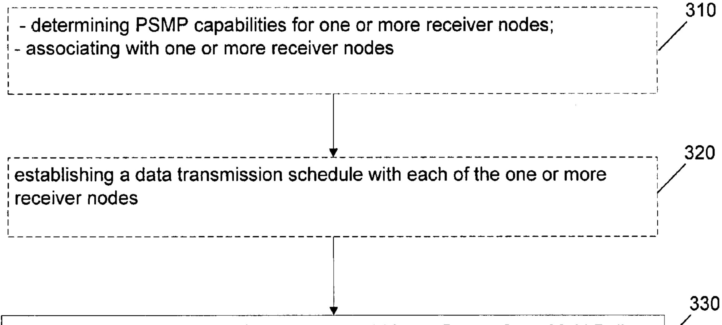
transmitting a management frame (e.g., an 802.11n Power Save Multi Poll (PSMP) frame) to identify a scheduled data transmission time and direction for each of one or more receiver nodes in a wireless network, the management frame including at least one multi-purpose field, the multi-purpose field to provide information related to a scheduled unicast data transmission and alternatively to identify a multicast address for a scheduled multicast data transmission
