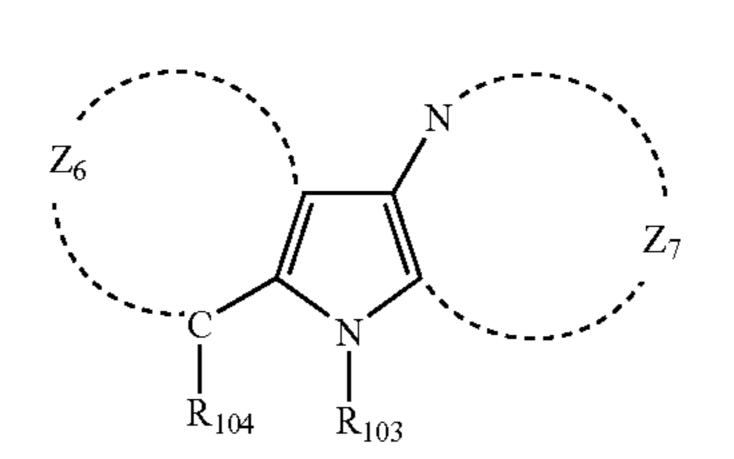
wherein R<sub>103</sub> represents an alkyl group which may have a substituent, a cycloalkyl group which may have a substituent, an aryl group which may have a substituent or a heterocyclic group which may have a substituent; R<sub>104</sub> represents a hydrogen atom or a substituent; and  $Z_6$  and  $Z_7$  each independently represents a pyridine ring.
