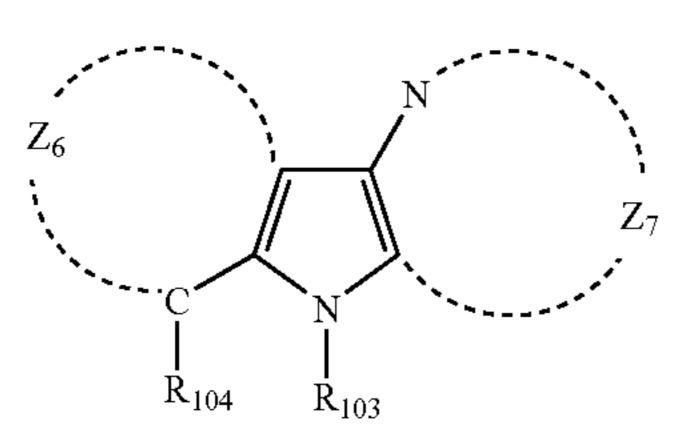
wherein  $R_{103}$  represents an alkyl group which may have a substituent, a cycloalkyl group which may have a substituent or a heterocyclic group which may have a substituent;  $R_{104}$  represents a hydrogen atom or a substituent; and  $Z_6$  and  $Z_7$  each independently represents an atom group which is necessary to form a 5-7 membered heterocylic ring containing nitrogen.
