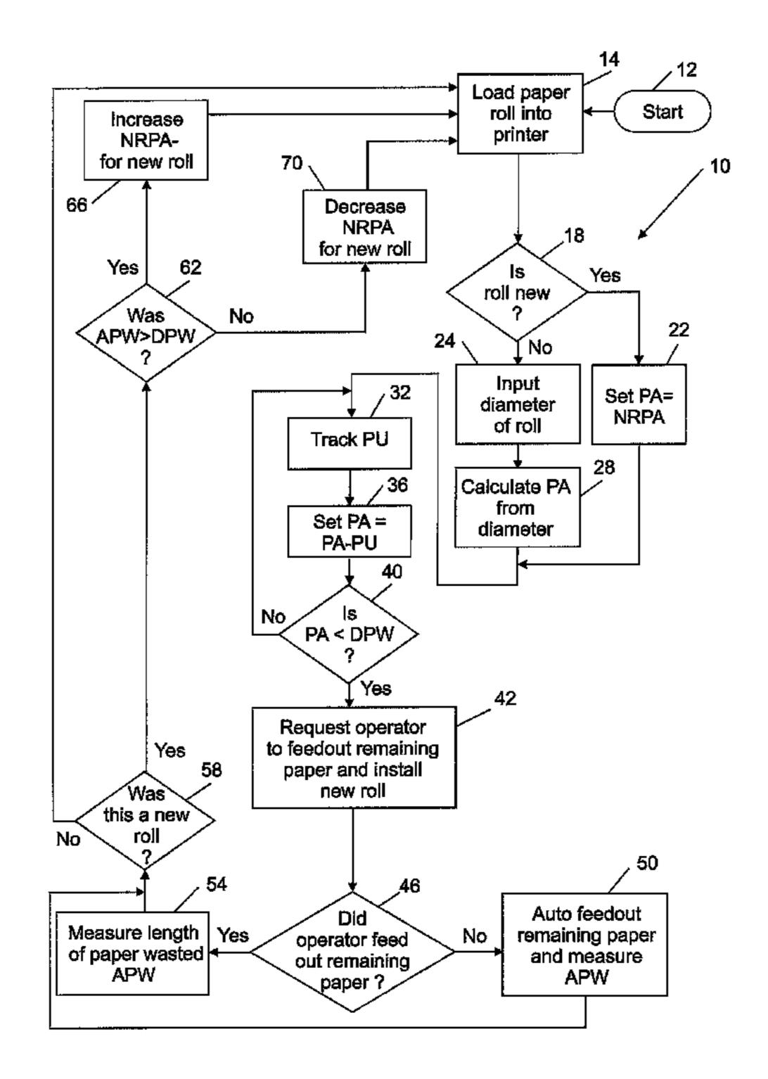
FIG. 1 Printer Paper Indexing Monitor Processor Memory
