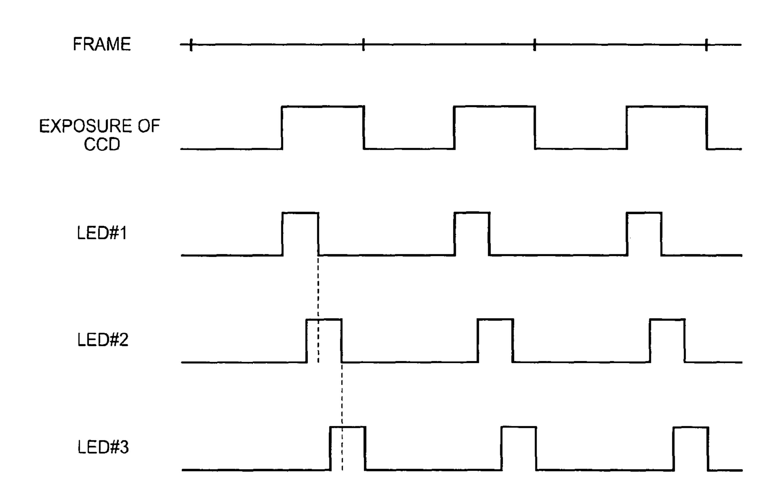
ILLUMINATION APPARATUS, IMAGING APPARATUS AND IRRADIATION METHOD FOR AN IMAGING APPARATUS COMPRISING LIGHT EMITTING DIODES WHICH ARE DUTY-DRIVEN DURING AN IMAGING PERIOD OF A FRAME PERIOD
