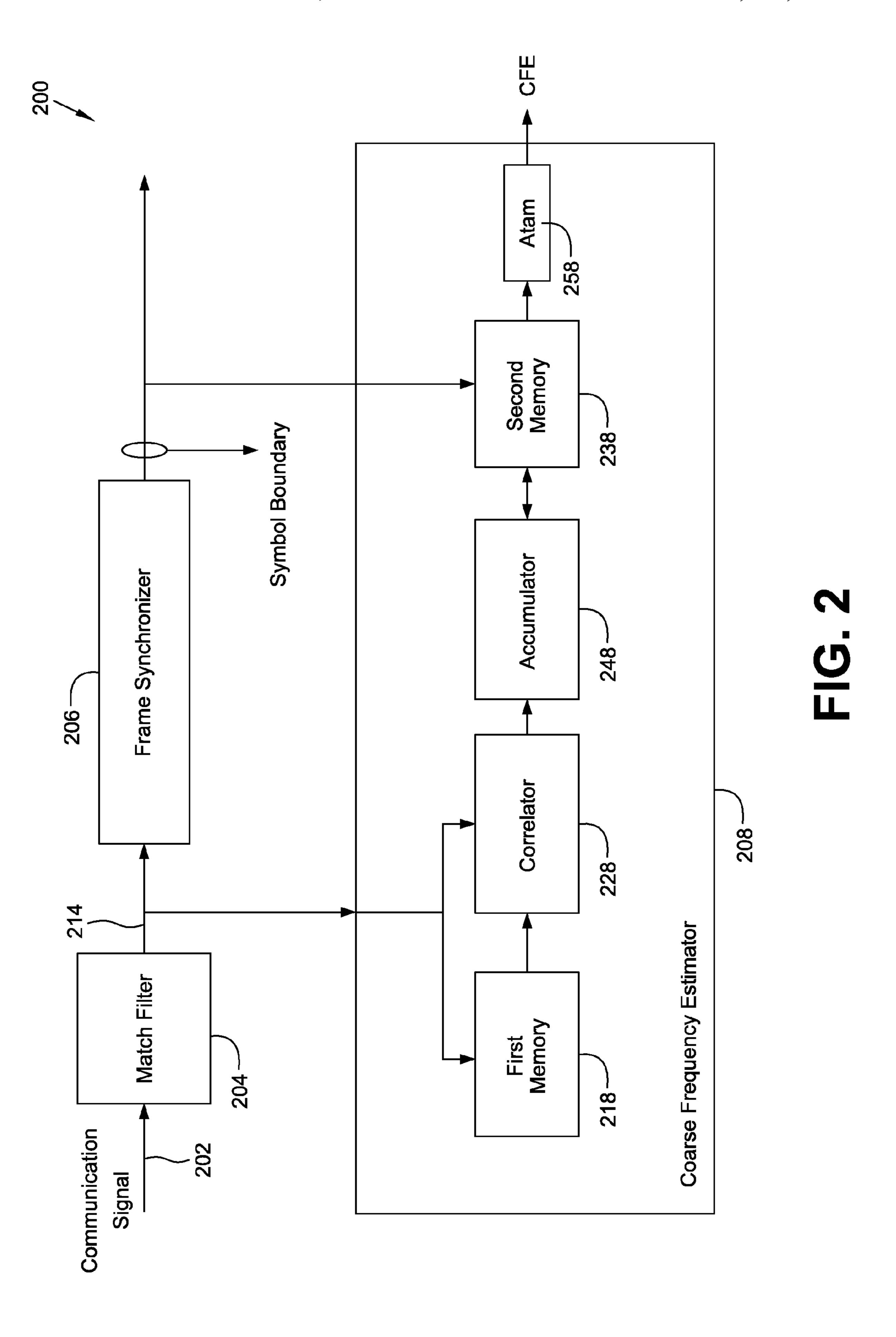
Select one of the metrics according to the symbol boundary to obtain a coarse frequency offset estimate
