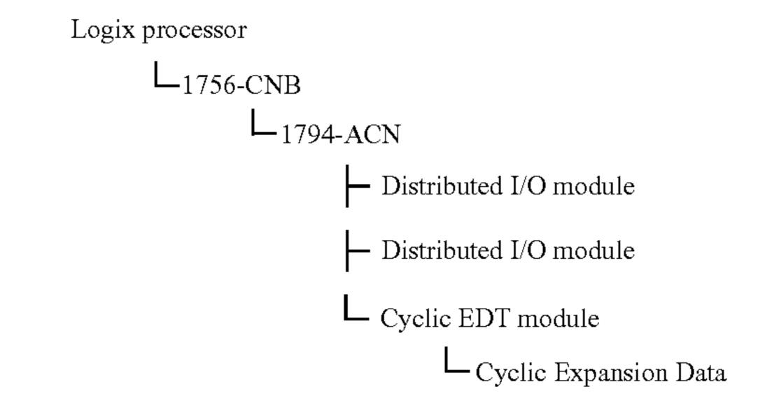
At this point the user can select the cyclic expansion data to view/modify the associated data and its RPI. It is assumed that a profile/applet for the associated Distributed I/O module with data extension will be need to place the expansion input and output data into the correct area/tags.
