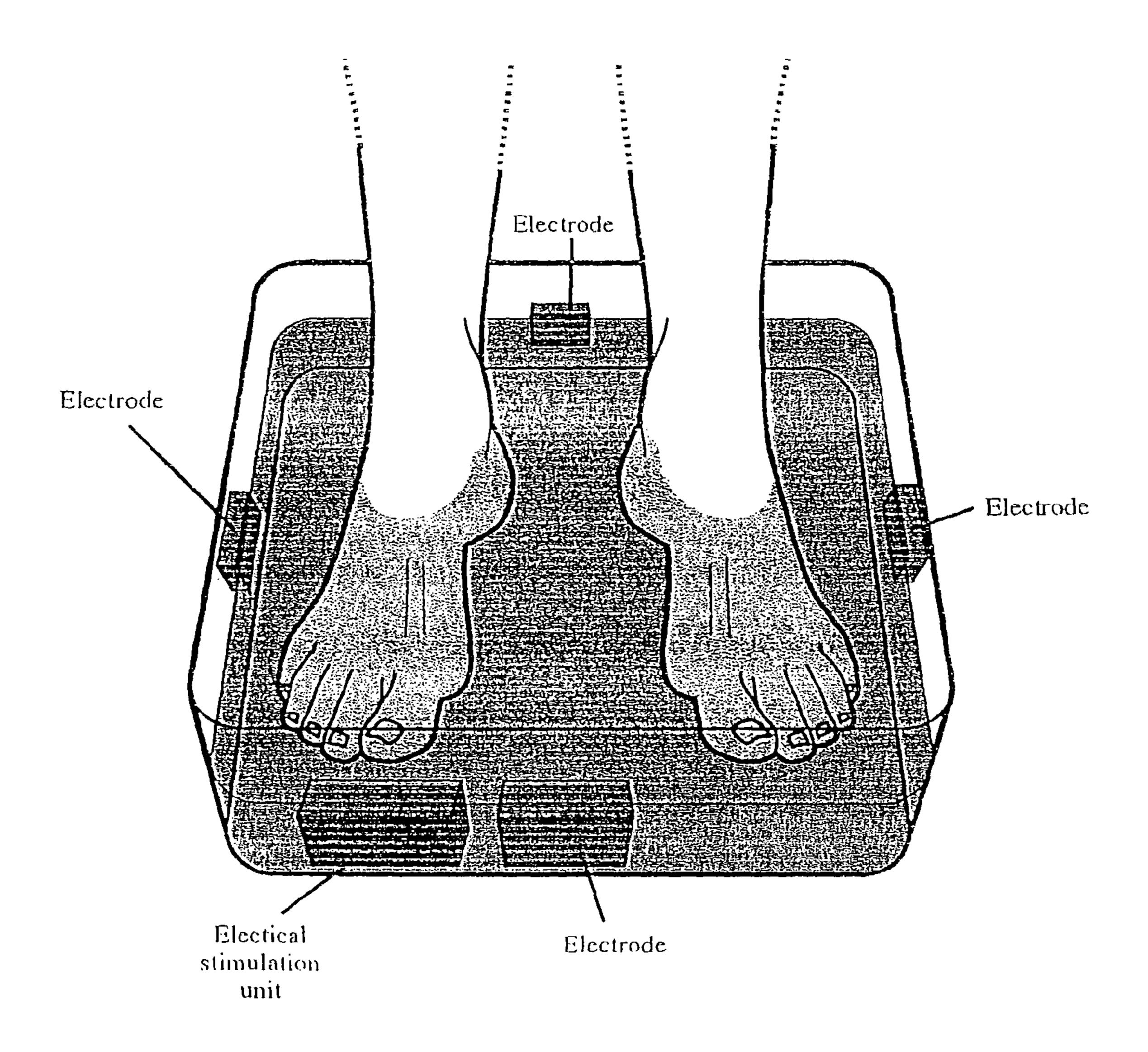
Figure 1. Electrical Stimulation Unit and Water Bath System
