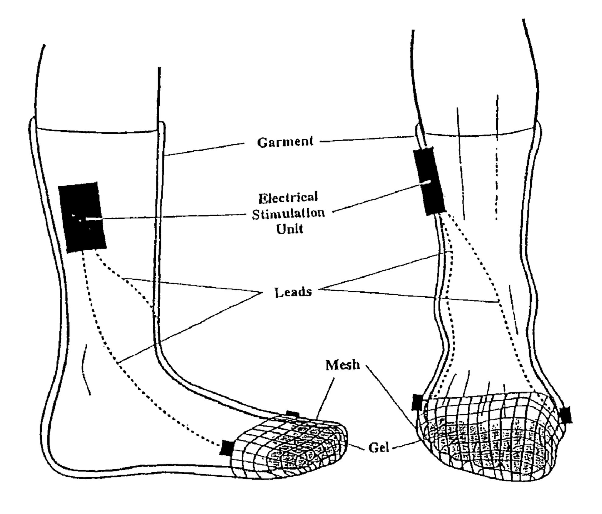
Figure 2: The Electrical Stimulation Unit and Garment System
