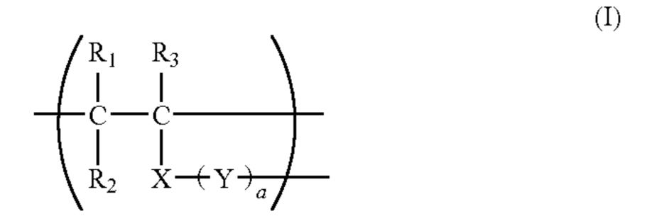
wherein R<sub>1</sub> to R<sub>3</sub> each independently represents hydrogen or a hydrocarbon group, R<sub>1</sub> may be bonded to R<sub>3</sub> to form a ring; X represents a connecting group having a valence of 3 or higher; Y may be the same or different and each represents a functional group which may have a halogen atom at a terminal thereof; and a is an integer of 2 or larger.
