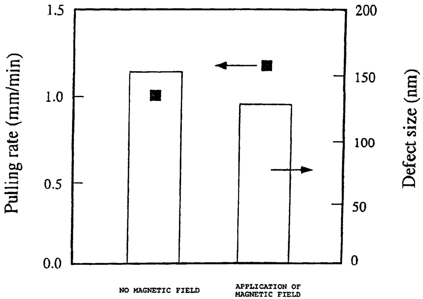
INFLUENCE OF MAGNETIC FIELD ON CRYSTAL GROWTH RATE AND DEFECT SIZE
