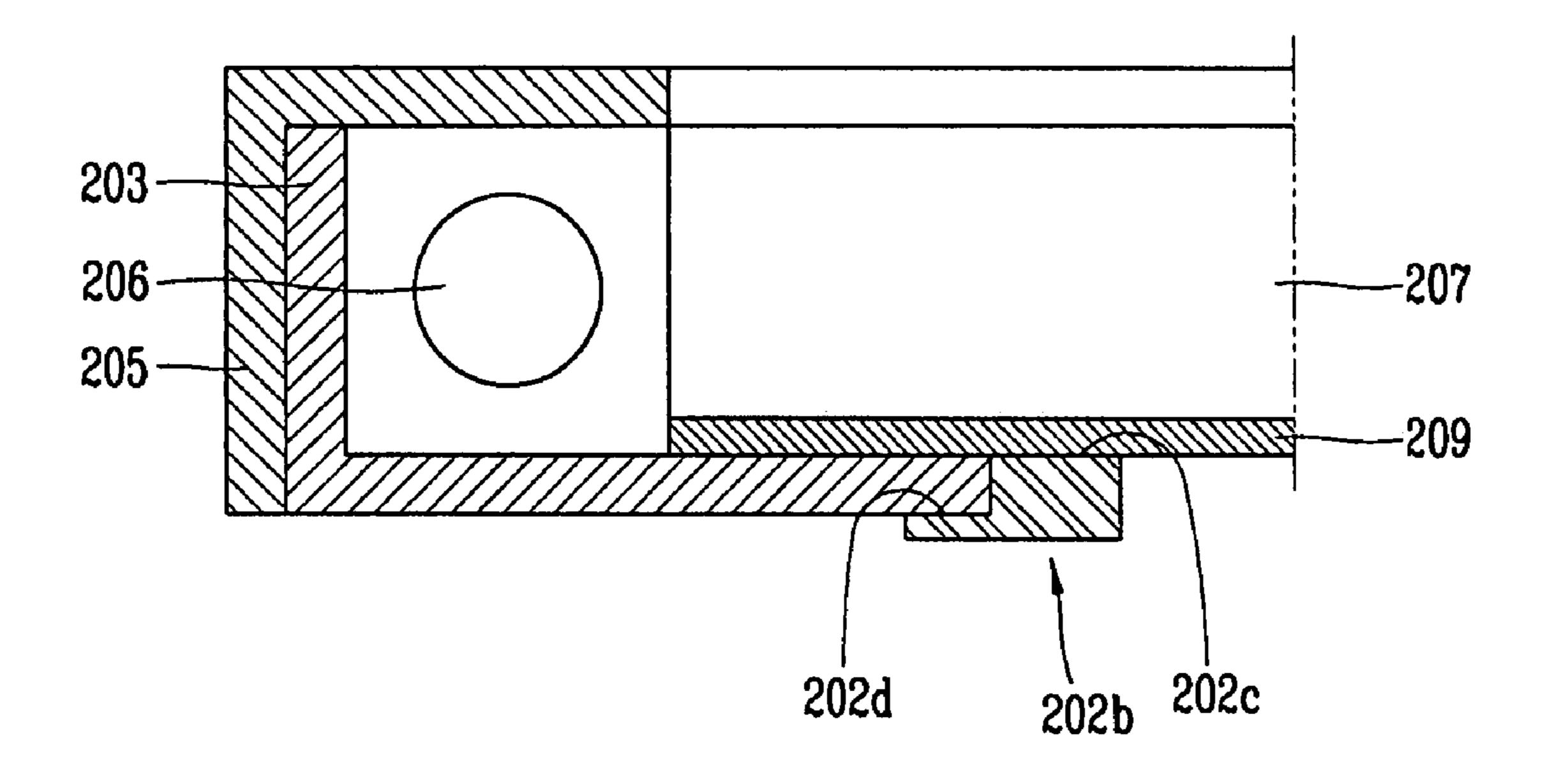
LIQUID CRYSTAL DISPLAY DEVICE WITH A MAIN SUPPORT FRAME HAVING SLIDE GROOVE PORTIONS THEREIN AND A FIRST UPPER COVER HAVING SLIDE PROTRUSIONS THEREIN INSERTED INTO THE SLIDE GROOVE PORTIONS, AND METHOD OF FABRICATING THEREOF
