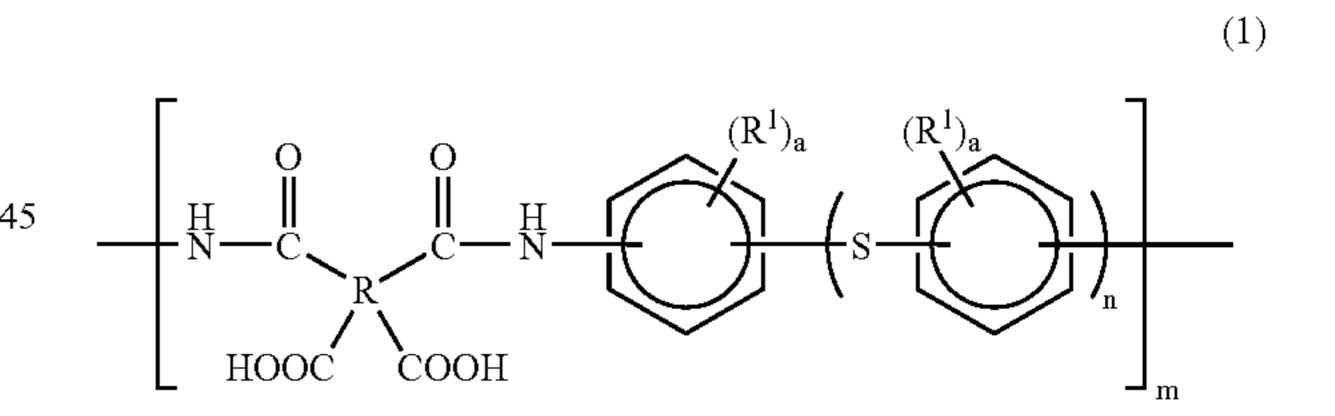
In the formula (1), R<sup>1</sup> is independently an alkyl group having 1 to 3 carbon atoms or a cyano group, and a is the number of substituent R<sup>1</sup> and independently an integer of 0 to 4. a is preferably 0 (namely, no R<sup>1</sup> is substituted), or R<sup>1</sup> is a cyano group and a is preferably 1.
