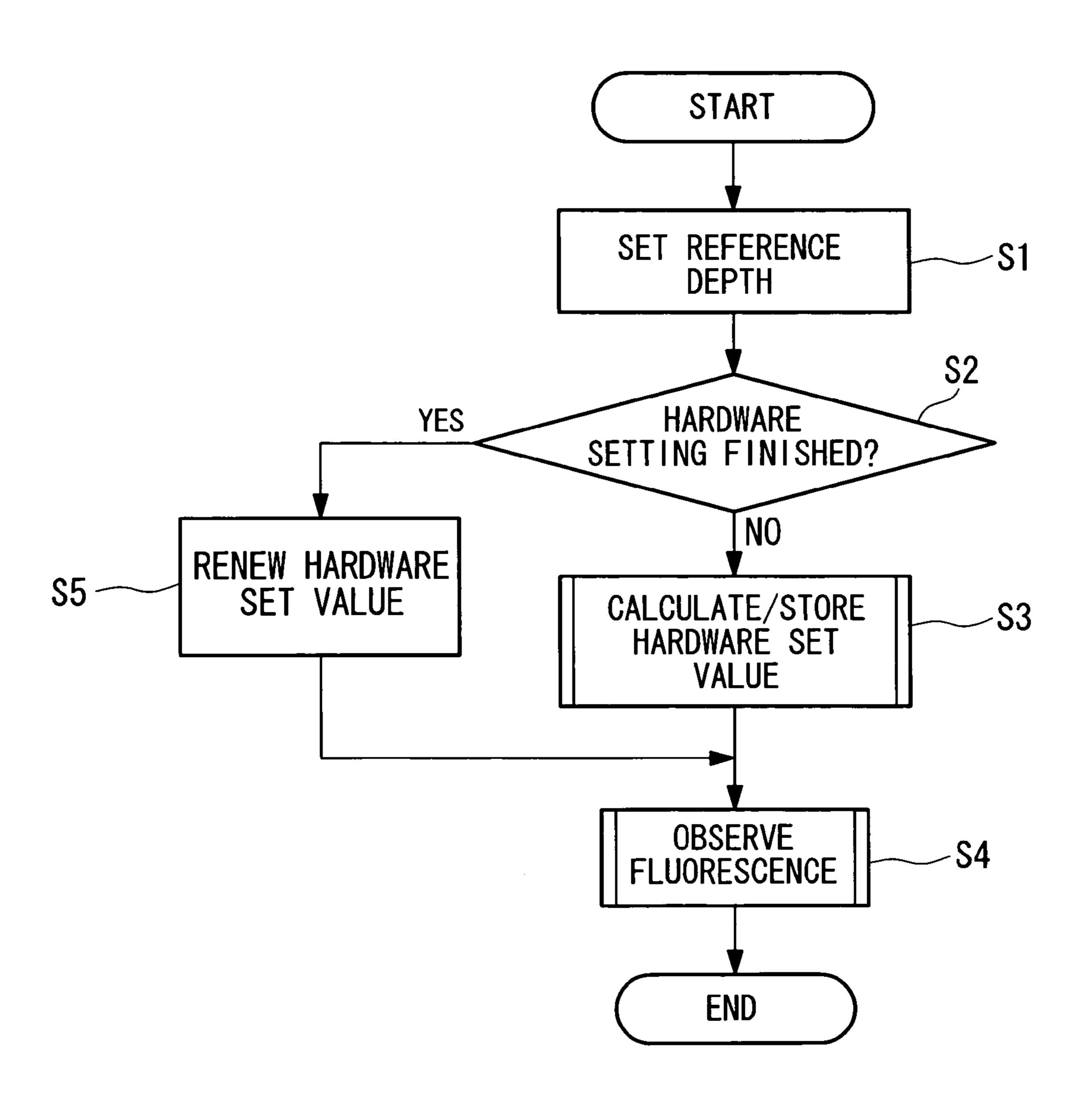
SCANNING OPTICAL DEVICE WHICH SETS HARDWARE IN ASSOCIATION WITH A DEPTH OF A FOCUS POSITION BASED ON HARDWARE SET VALUES STORED IN ASSOCIATION WITH DEPTHS OF FOCUS POSITIONS
