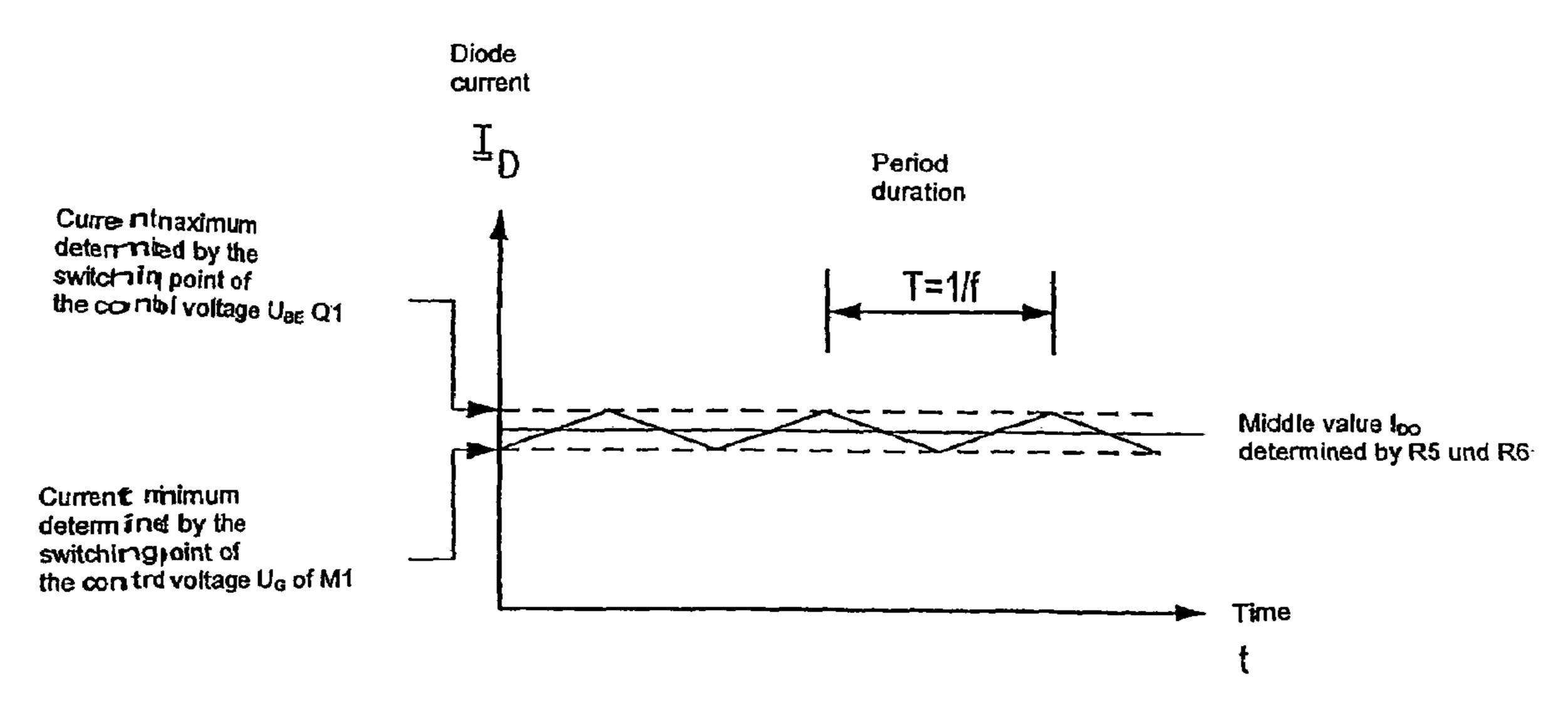
Frequency: f < 100 kHz (determined by UNETZ and suitable dimensioning of L1 and the switching thresholds for the control voltages UBE and UG of the power transistors Q1 and M1)
