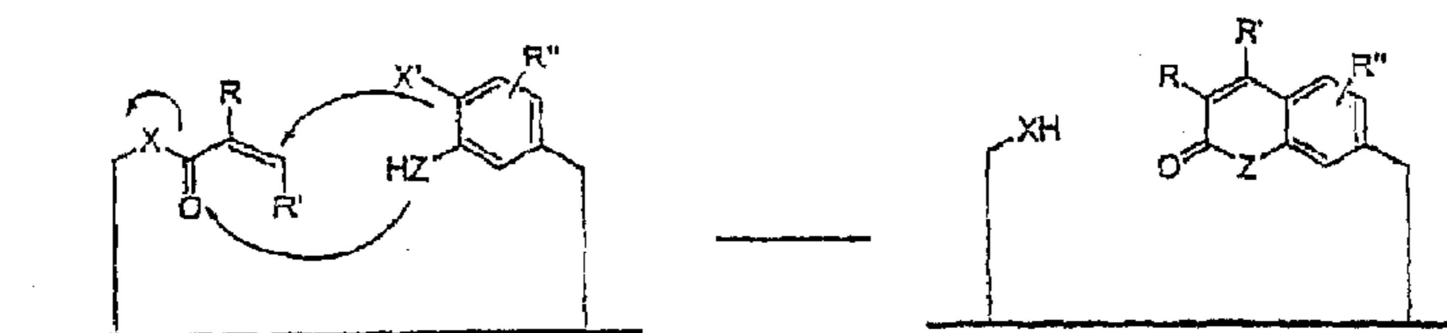
FIG. 6G. Acylation Coumarine or quinolinon formation by a Heck reaction followed by a nucleophilic substitution
