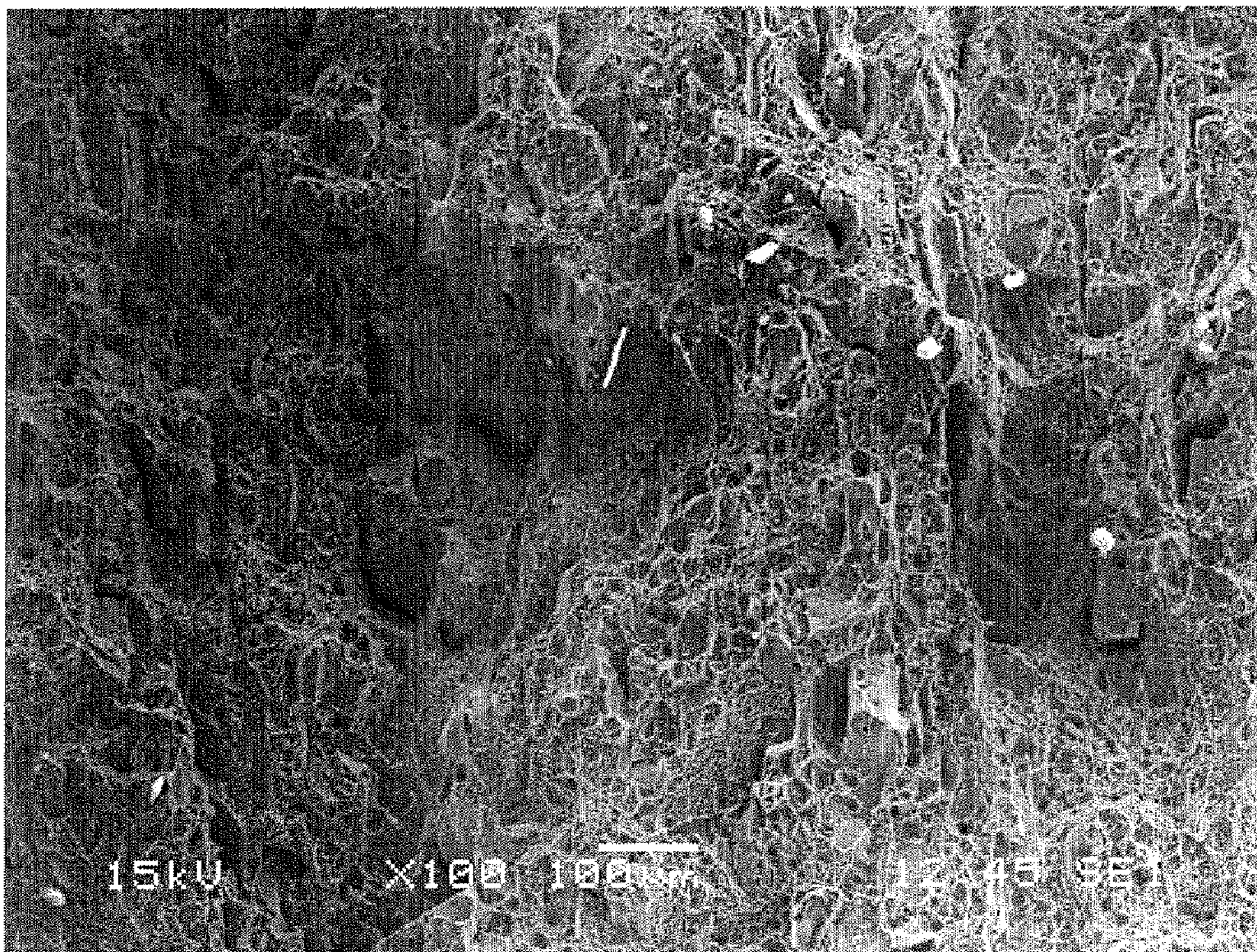
Figure 2. Fractography of B sample tested at -65F (showing many areas with brittle fracture mode)
