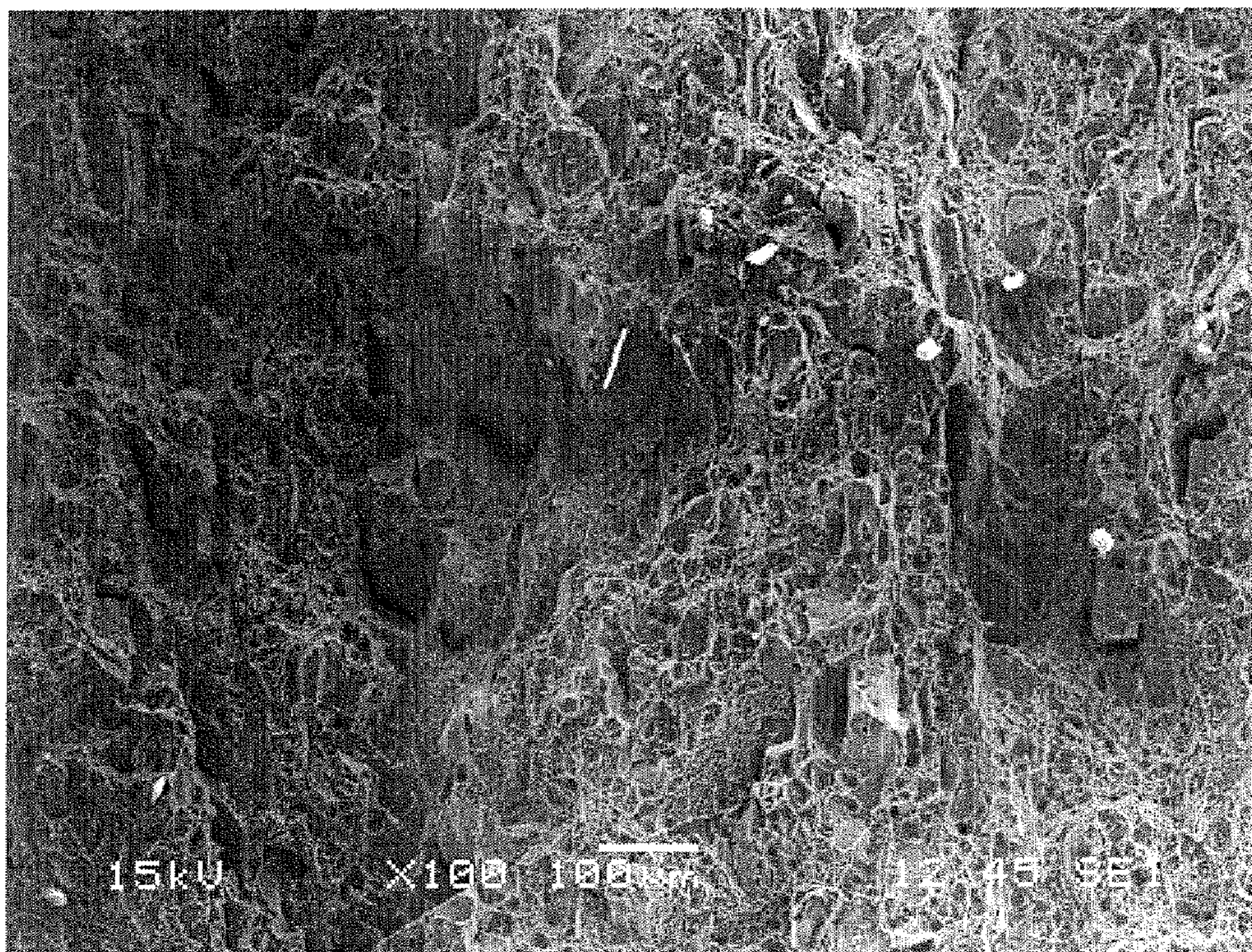
Figure 2. Fractography of B sample tested at -65F (showing many areas with brittle fracture mode)
