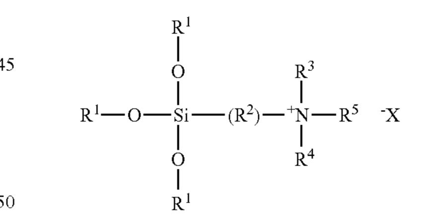
wherein  $R^1$ =hydrogen and/or  $C_1$  to  $C_4$  alkyl;  $R^2$ =divalent hydrocarbon radical with  $C_1$  to  $C_8$  carbon atoms,  $R^3$ =hydrogen to  $C_1$  to  $C_4$  alkyl,  $R^4$ =hydrogen or  $C_1$  to  $C_{10}$  alkyl,  $R^5 = C_{10}$  to  $C_{22}$  saturated or unsaturated hydrocarbon radical and X=halide, carboxylate, sulfonate, hydroxide, sulfate, or phosphate,
