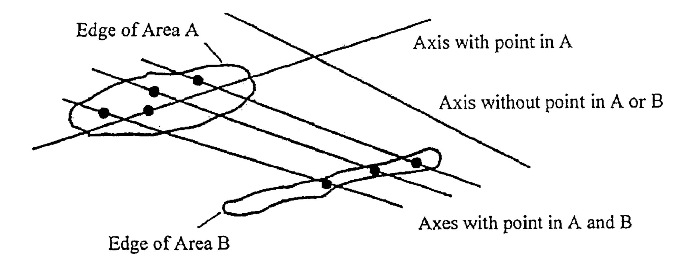
Intersecting points between the axes and the area
