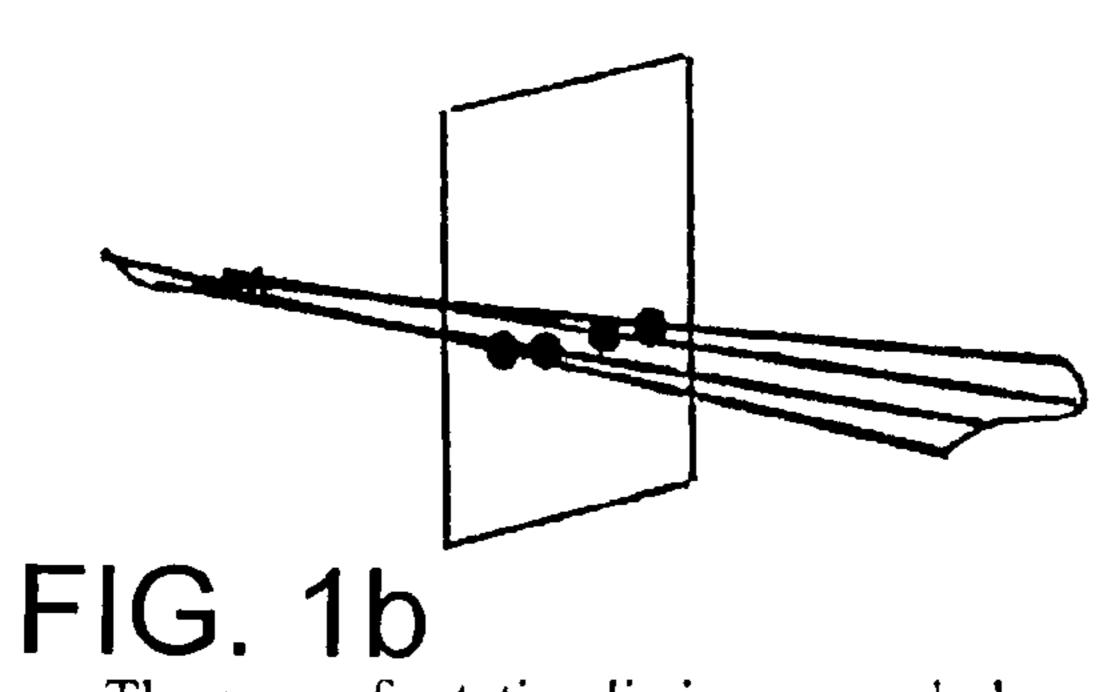
The axes of rotation lie in a curved plane and intersect the sagittal projection plane
