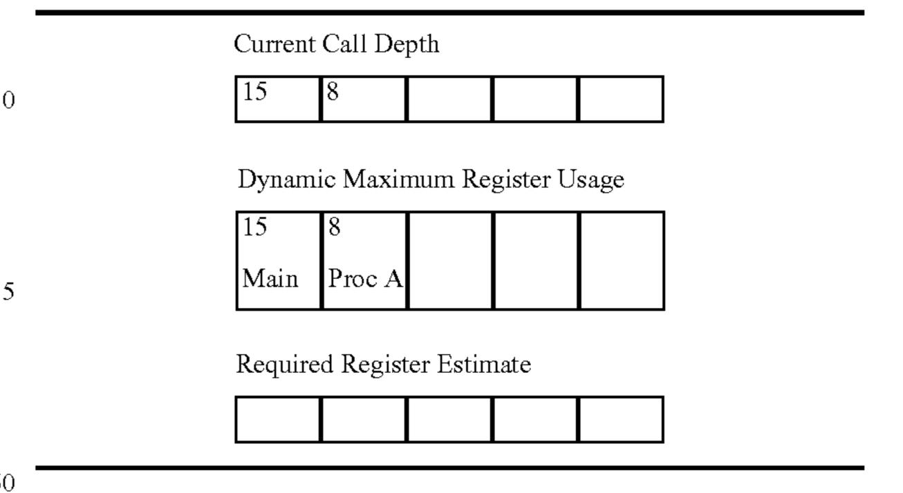
On entering procedure B, six registers are allocated, the value added to the CCD list and added to each of the predecessors in the list. The value is placed in the first free element in the DMRU list along with the procedure name. The predecessors in the DMRU list are also updated with the new maximums from the CCD list as shown below:
