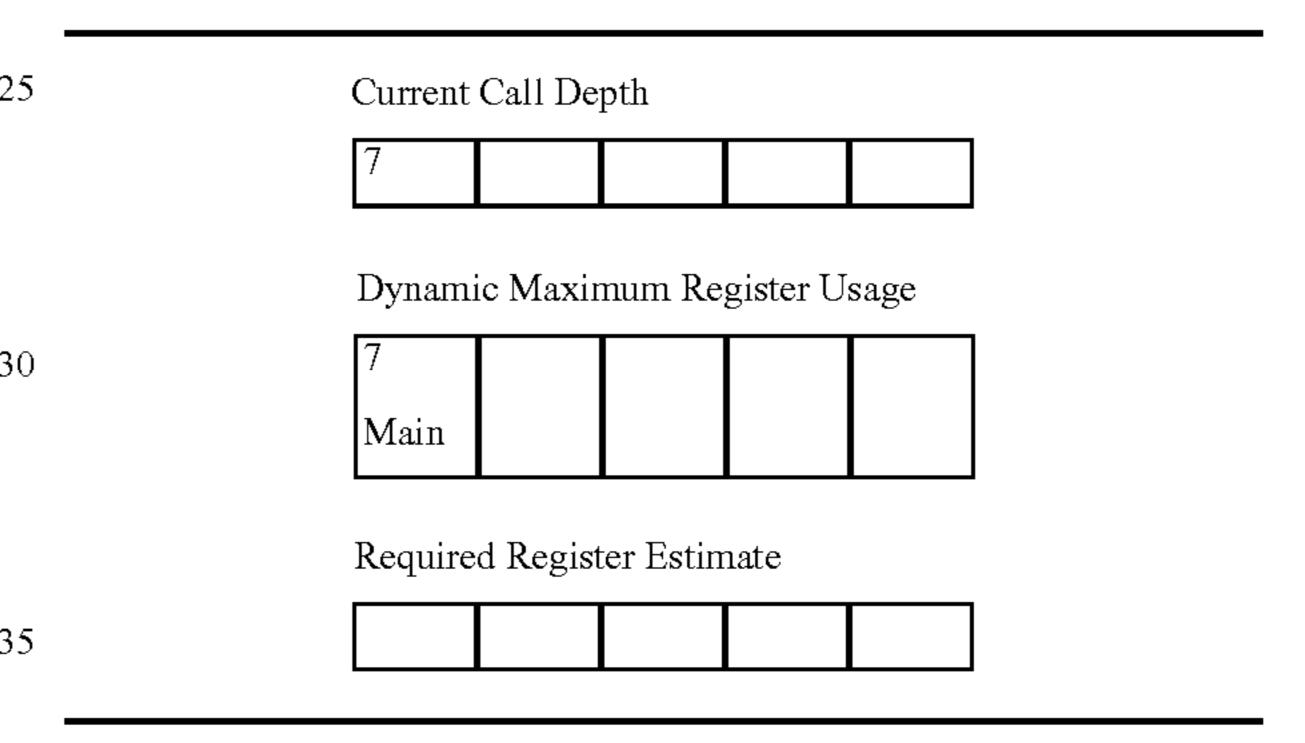
On entering procedure A, a further alloc instruction is processed which allocates eight registers to the procedure.
