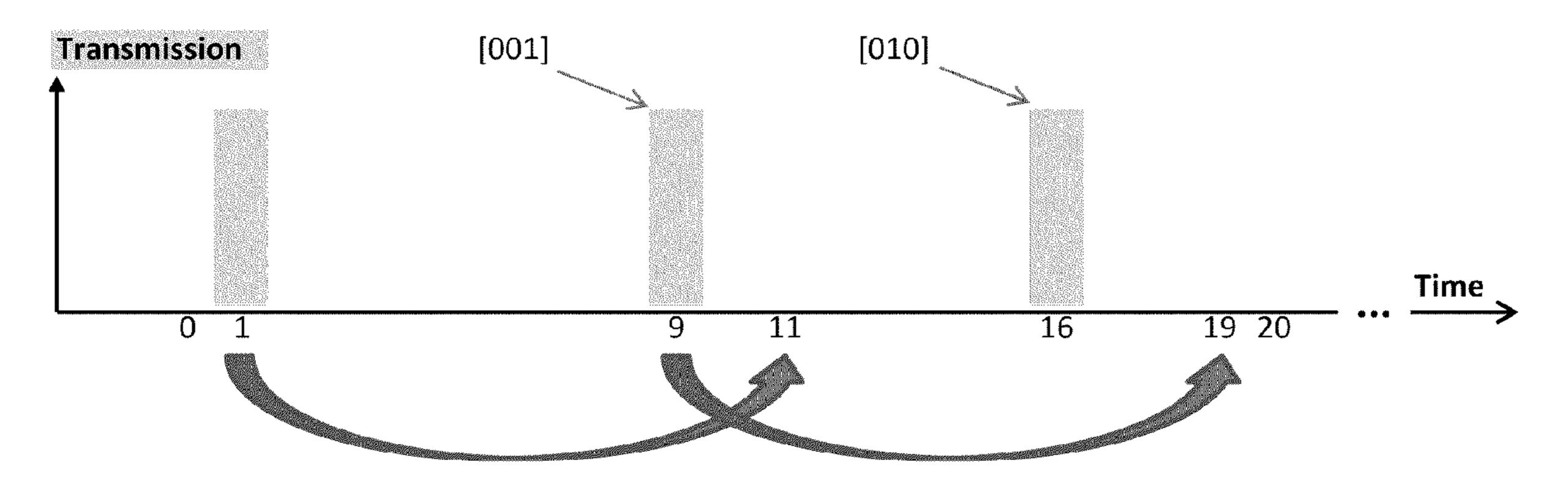
Figure 4 – Transmission Timing Randomization (permutation)
