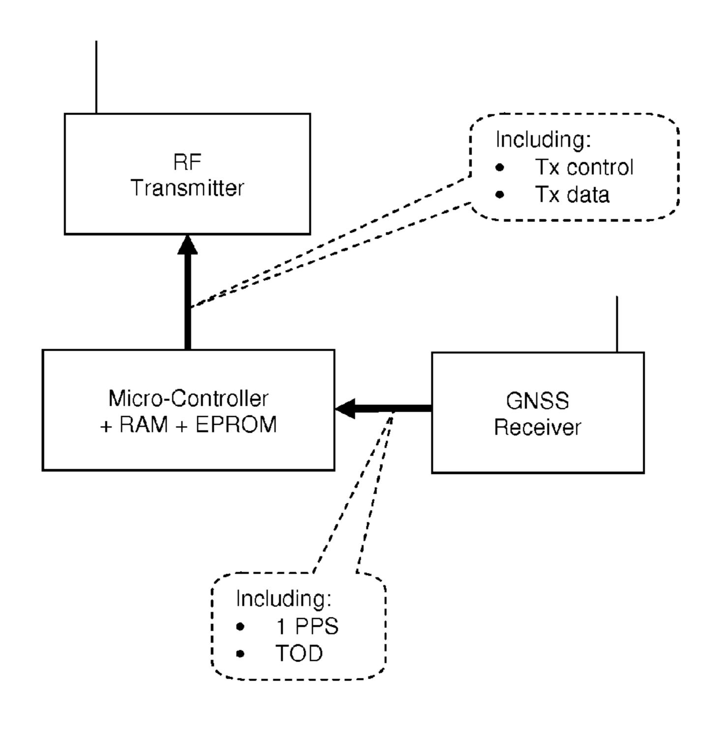
Figure 1 – Transmission Timing Modulation
