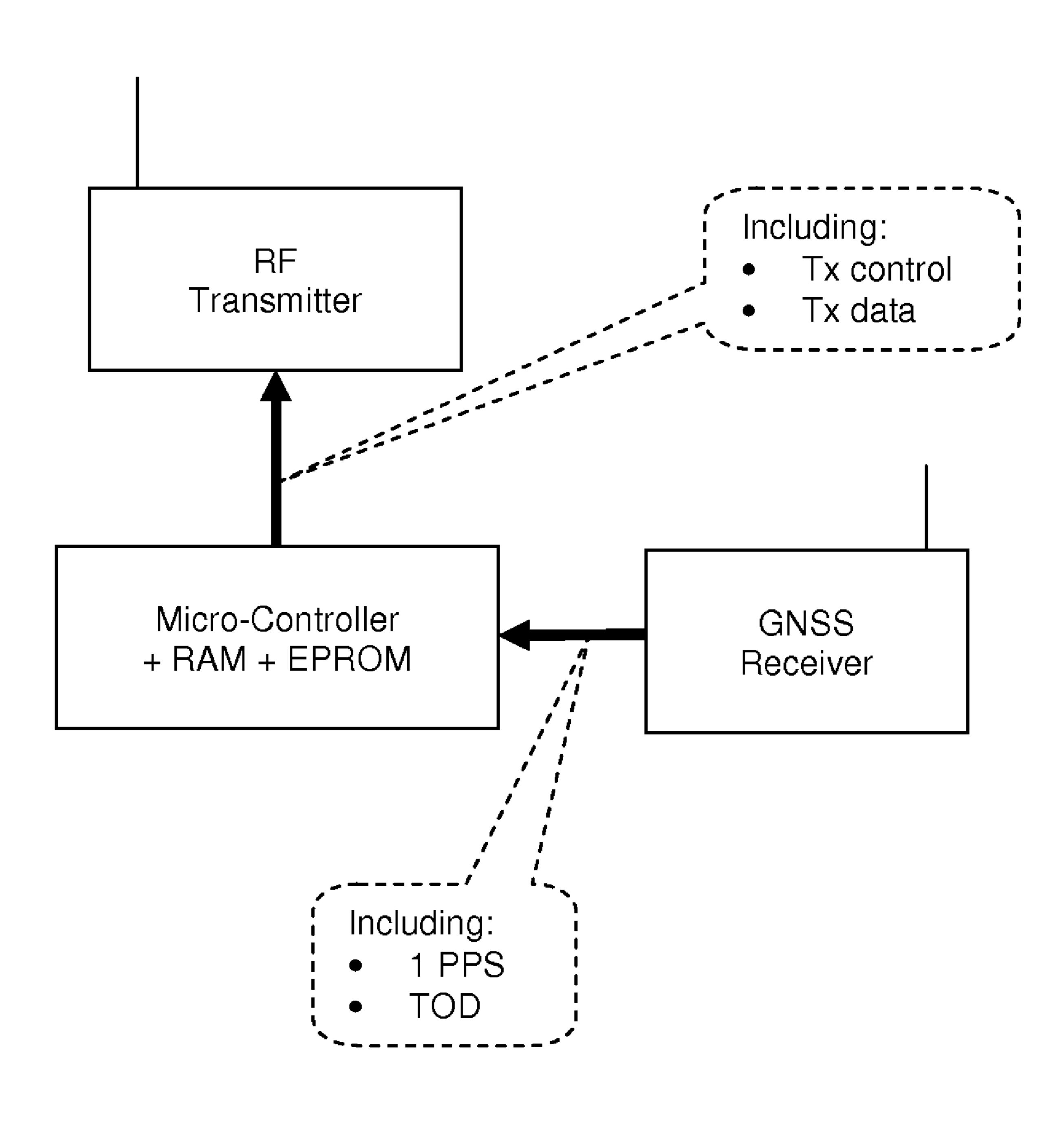
Figure 7 – Receiver Block Diagram
